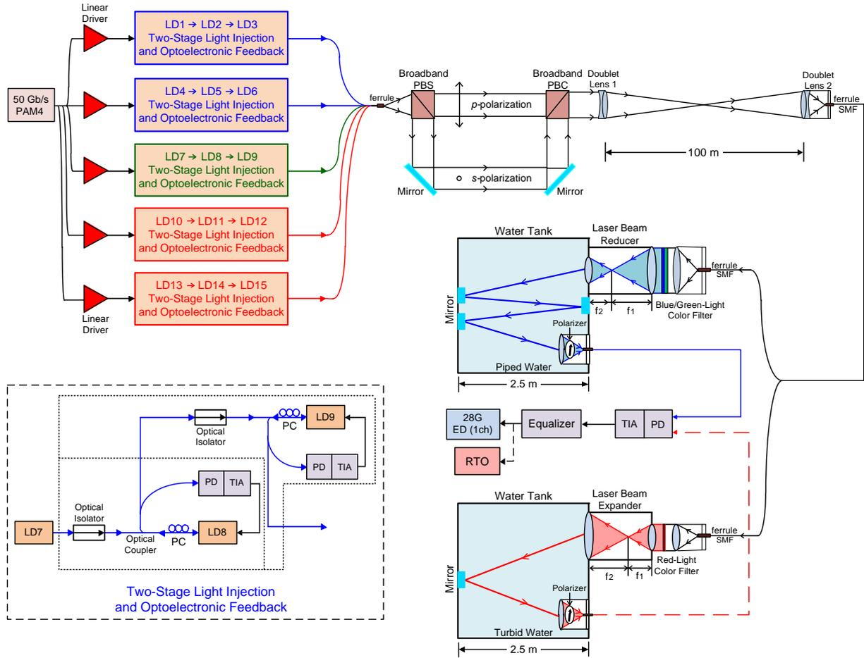
**Fig. 1.** The configuration of the illustrated 500 Gb/s PAM4 FSO-UWLT integration with a R/G/B five-wavelength polarization-multiplexing scenario over a 100-m free-space transmission with either 10-m piped underwater channel or 5-m turbid underwater channel.
