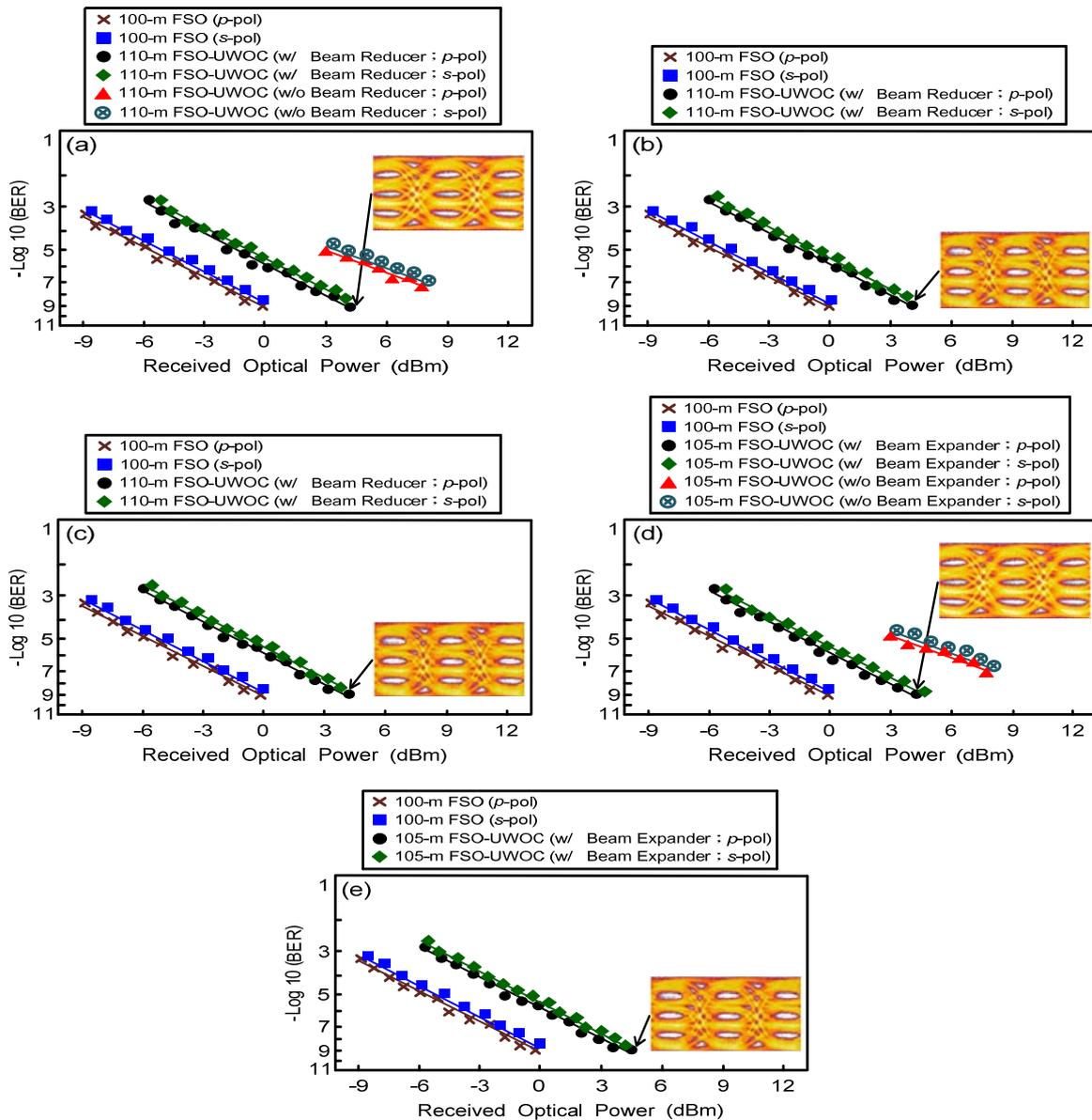
**Fig. 2.** The BER performances of 50 Gb/s PAM4 signal at a selected wavelength of (a) 450.6 nm (b) 488.2 nm, (c) 520.4 nm, (d) 642.6 nm, and (e) 660.3 nm in the scenarios through a 100-m free-space transmission ( $p$ - and  $s$ -polarizations) and that through a 100-m free-space transmission with either 10-m piped underwater link or 5-m turbid underwater link ( $p$ - and  $s$ -polarizations).
