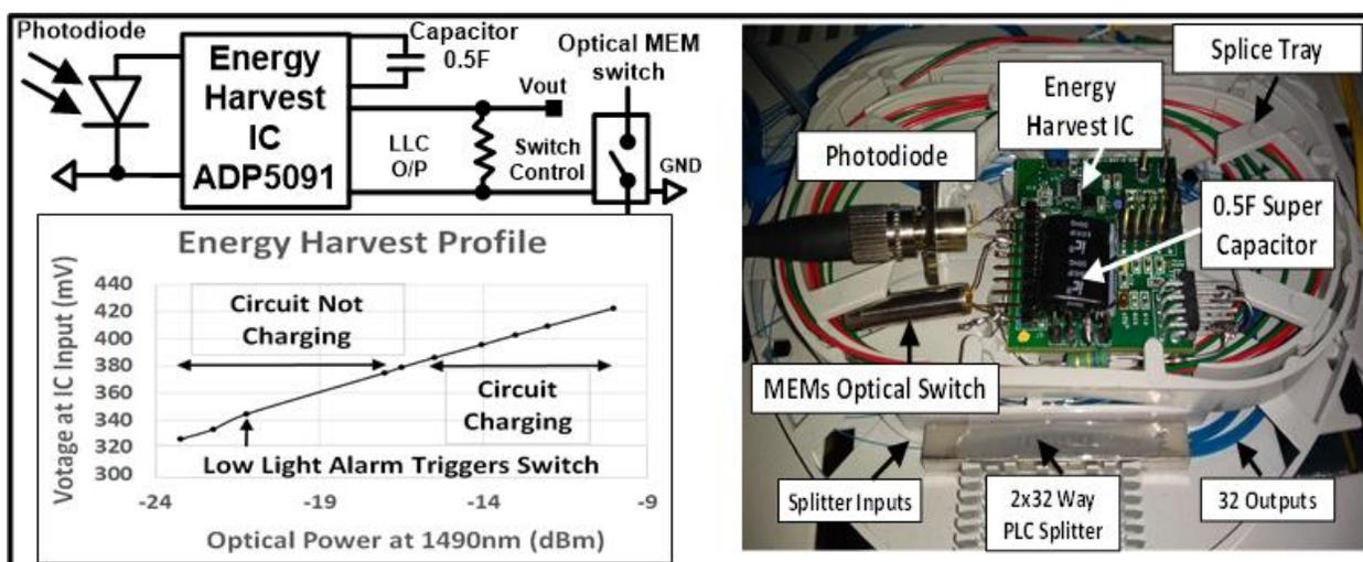
Figure 2. Circuit Diagram & measured harvest power profile Figure 3. Circuit in Splice tray with 2x32 splitter
