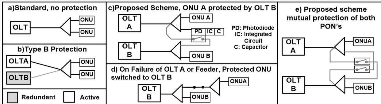
Figure 1 a) Unprotected PON; b) Standardized Type B configuration; c) Proposed new scheme single protection during working condition; d) Proposed new scheme single protection during failure condition; e) Mutual protection
