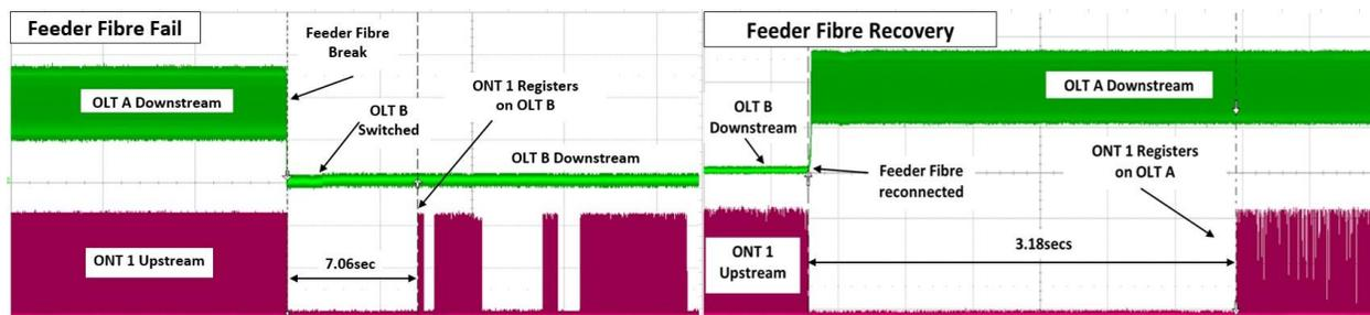
Figure 7. RTO Measurement of loss and recovery after the feeder is pulled from OLT A (left) and reinserted (right).
