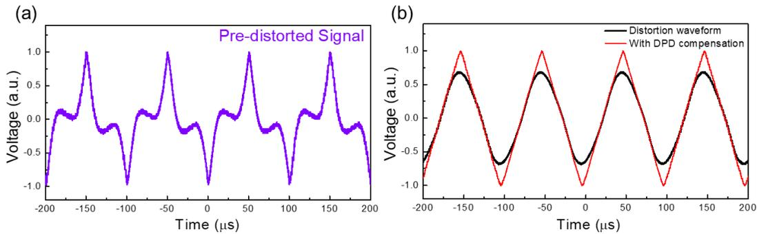
Fig. 2. (a) Designed pre-distorted signal for 10 KHz distorted triangular waveform. (b) Measured signals with and without DPD compensation.
