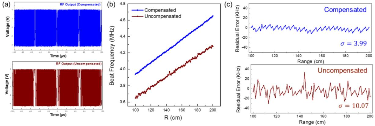
Fig. 4. FMCW LiDAR ranging experiment results for compensated and uncompensated frequency modulation. (a) Images of RF output signal from real-time scope. (b) Beat frequency for the distance from 1 m to 2 m in air. (c) The beat frequency residual error.
