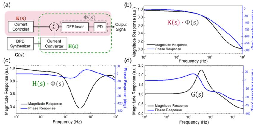
Fig. 1. (a) Block diagram of the DPD frequency compensation method. (b) Frequency response of  $K(s) \cdot \Phi(s)$ . (c) Frequency response of  $H(s) \cdot \Phi(s)$ . (d) DPD synthesizer frequency response  $G(s)$ .
