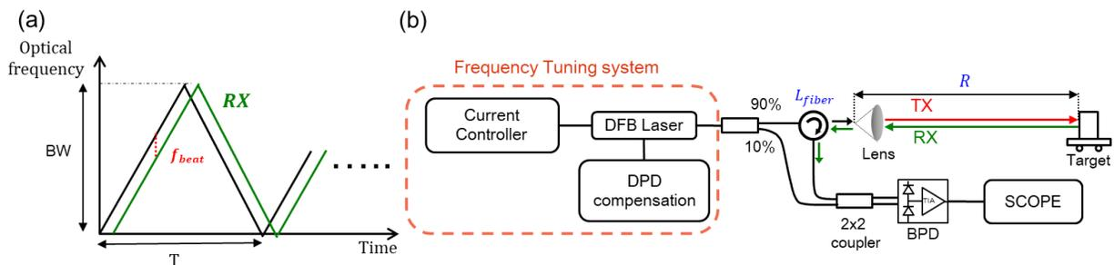
Fig. 3. (a) Concept of FMCW LiDAR with triangular modulation. (b) The measurement setup of FMCW LiDAR ranging system.
