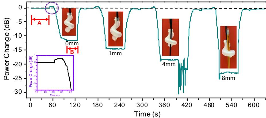
Figure 3: Real-time monitoring of the twining plant inspired spiral gripper using optical power measurement of the embedded high-birefringence fiber optic sensor.
