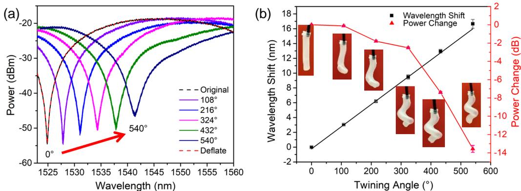
Figure 2: (a) Interference optical spectra of the embedded high-birefringence fiber sensor in the spiral gripper; (b) Relationship between twining angle and wavelength shift (black) and power change (red).
