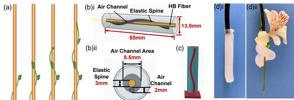
Figure 1: (a) Illustration of the wrapping motion in a twining plant; (b)i. 3D view of the twining plant inspired soft robotic spiral gripper with embedded high-birefringence (HB) fiber optic sensor; ii. Cross-section view of the spiral gripper; (c) 3D printed molds for fabricating the spiral gripper; (d)i. Photo of the robotic spiral gripper before actuation; ii. Photo of the robotic spiral gripper after actuation and twining around a flower stem.
