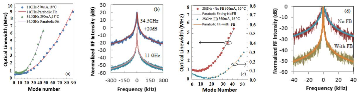
Fig. 2. Measured laser mode optical linewidths vs. mode number and parabolic fits for 11 and 34.5GHz (a) and 25GHz with and without external feedback cavity (FB) (c) QD CCL by using OEwaves OE4000 automated laser linewidth/phase noise measurement system. Normalized first harmonic RF spectra with related Lorentzian fits for 11 and 34.5GHz (b) and 25GHz with and without external feedback cavity (FB) (d) QD CCL measured by using Keysight Technologies N9030A 50 GHz PXA signal analyzer at RBW=100Hz.
