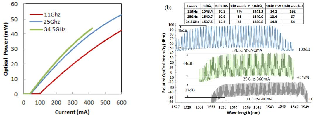
Fig. 1. (a) Light-current characteristics (b) Optical spectra of 11, 25 and 34.5 GHz QD CCL measured by Anritsu MS9740A optical spectrum analyzer at 0.01 nm resolution. Inset: a table of central wavelength, optical bandwidth, and mode number at 3dB and 10 dB of three QD CCLs.
