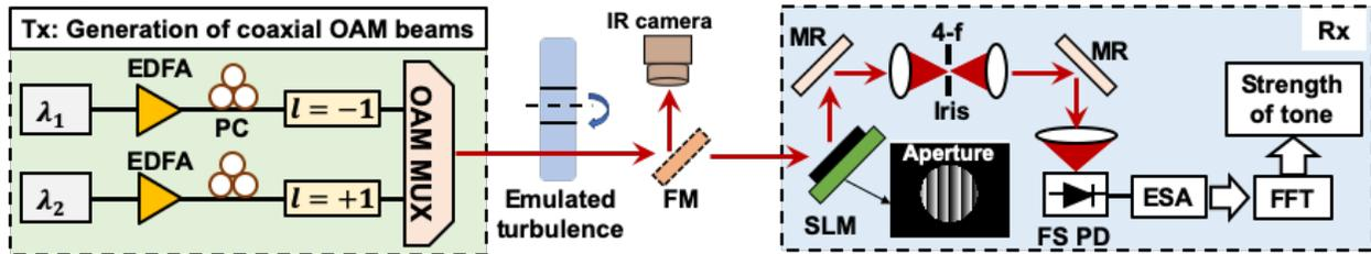
Figure 2. Experimental setup of monitoring the misalignment of an FSO link under turbulence effects: the OAM beams are transmitted separately through the emulated turbulence effects. The beating strength of OAM  $l = \pm 1$  beams is used to estimate the Rx misalignment. EDFA: erbium-doped fiber amplifier; PC: polarization controller; SLM: spatial light modulator; FM: flip mirror; IR: infrared; FS PD: free space photodetector.
