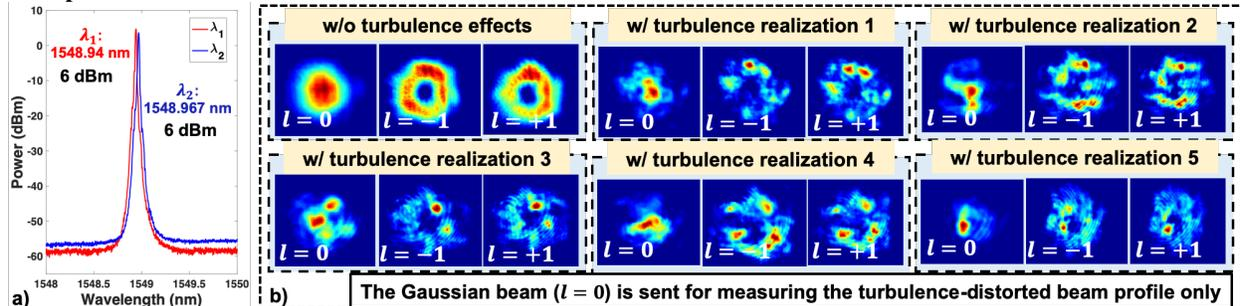
Figure 3. a) Measured optical spectrum of two laser sources around 1550 nm; b) Measured intensity profiles for Gaussian ( $l = 0$ ) and OAM  $l = \pm 1$  beams under effects of 5 different turbulence realizations: each beam is sent one at a time. The Gaussian beam is transmitted for beam profile measurement only (to indicate the turbulence distortions) and the two OAM modes would be sent simultaneously for alignment monitoring.
