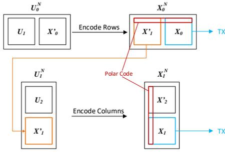
Fig. 1: Encoding process.
