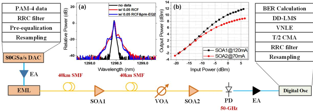
Fig. 1. Experimental setup of the EML-based IM/DD 100Gbit/s/λ PAM-4 signal transmission at O-band: (a) spectra of the modulated optical signal (0.02nm); (b) output power curves vs. input power for SOA1 and SOA2.
