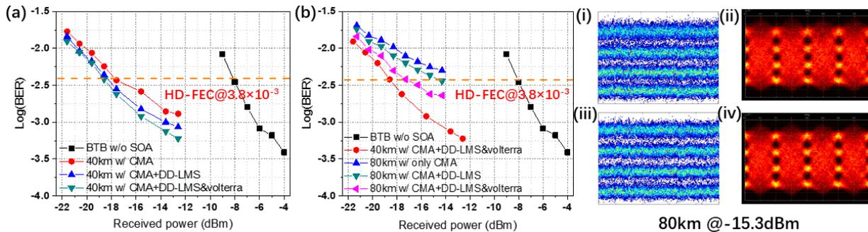
Fig. 3. The measured BER curves versus received optical power after (a) 40-km and (b) 80-km SSMF transmission; the constellation (i) and eye diagram (ii) with only linear equalization; the constellation (iii) and eye diagram (iv) with linear and nonlinear equalization
