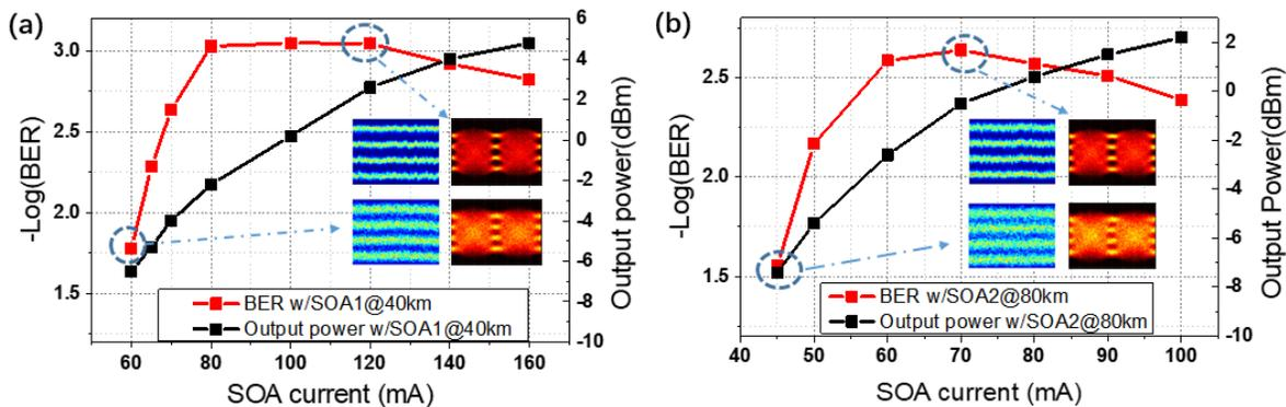
Fig. 2. The measured BER and output power versus SOA current: (a) after 40-km transmission with SOA1; (b) after 80-km transmission with SOA1 and SOA2.
