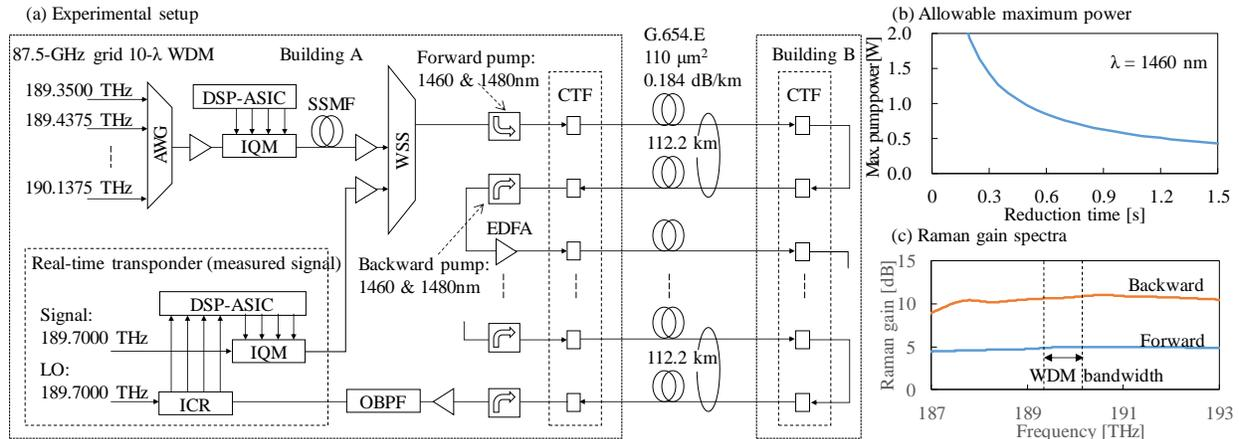
Fig. 2. (a) Setup for field experiments over G.654.E link, (b) Allowable maximum power as function of auto power reduction time, and (c) Raman gain spectra.
