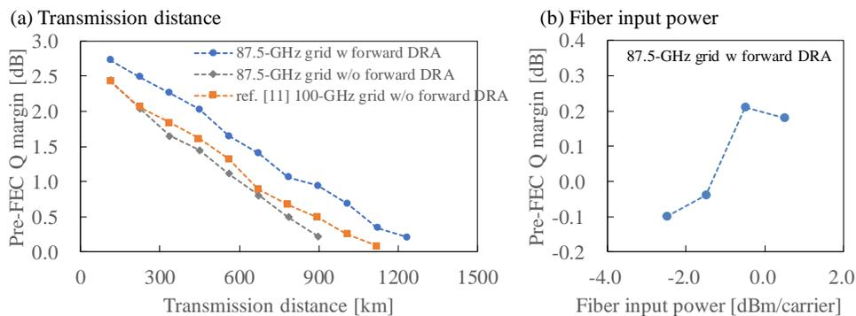
Fig. 3. Experimental results of pre-FEC Q margin of 500-Gb/s transmission using EDFA, backward DRA, with and without forward DRA (a) as function of transmission distance, (b) optimum fiber input power for the transmission distance of 1234.2km with forward DRA.
