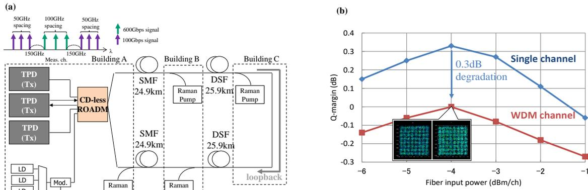
Fig. 2. (a) Field setup for 600-Gbps/lambda WDM transmission, (b) Experimental results.
