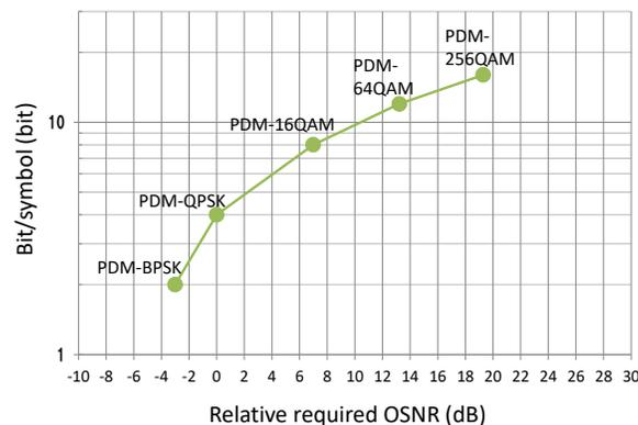
Fig. 1. OSNR requirements for high order modulation.
