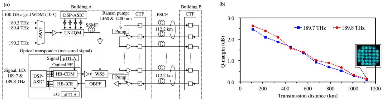
Fig. 3. (a) Field setup for 500-Gbps/ $\lambda$  WDM transmission, (b) Experimental results.
