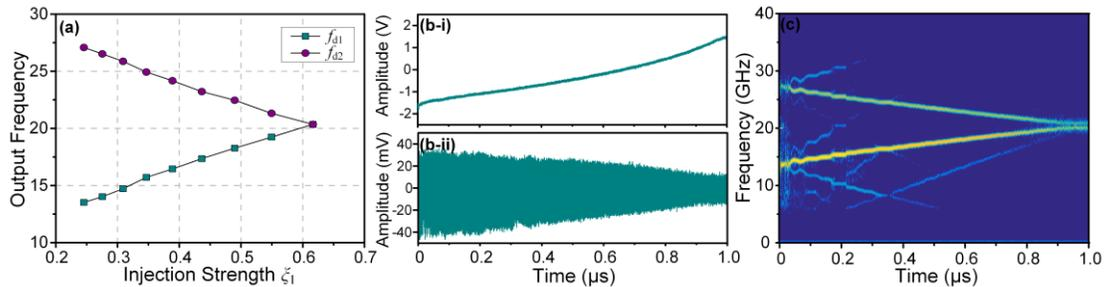
Fig. 3. (a) Frequencies of the generated microwave signals as a function of  $ML_1$ 's injection strength, (b) measured waveform of the control signal (i) and the generated DCMW (ii) with one period, and (c) instantaneous frequency-time diagram.
