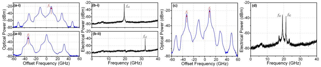
Fig. 2. Optical (a & c) and electrical (b & d) spectra of the SL subject to single-beam (a & b) and dual-beam (c & d) injection.
