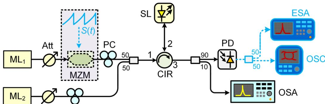
Fig. 1. Block diagram of the experimental set-up. ML: master laser, Att: optical attenuator, PC: polarization controller, MZM: Mach-Zehnder modulator,  $S(t)$ : control signal, CIR: optical circulator, SL: slave laser, PD: photodetector, OSA: optical spectral analyzer, ESA: electrical spectral analyzer, OSC: oscilloscope.
