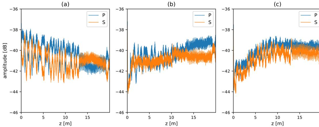
Fig. 2: Rayleigh scattering traces. Figure (a): same-core. Figure (b): cross-core 1. Figure (c): cross-core 2.
