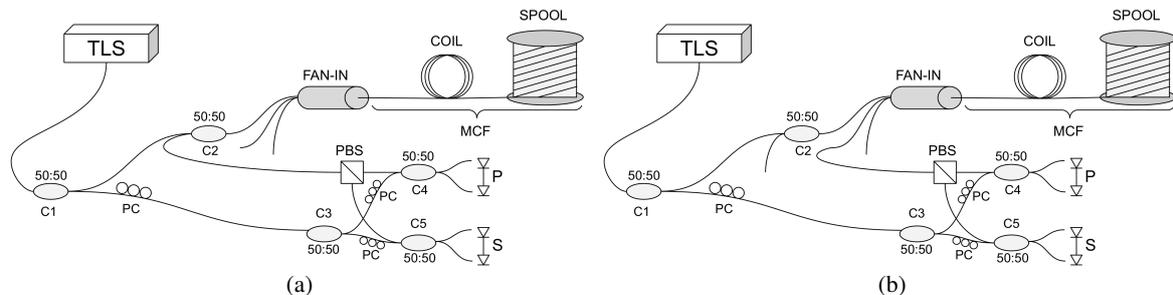
Fig. 1: Experimental setup. Figure (a): setup for the same-core measurement. Figure (b): setup for the cross-core measurement. TLS: tunable laser source; PC: polarization controller.
