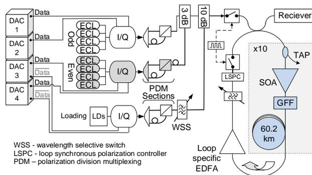
Fig. 1: 60.2km circulating loop test bed schematic
