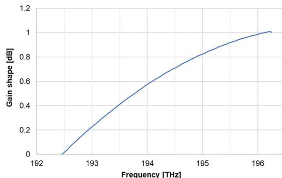
Fig. 2: Average gain shape of the SOAs with 60.2km spans
