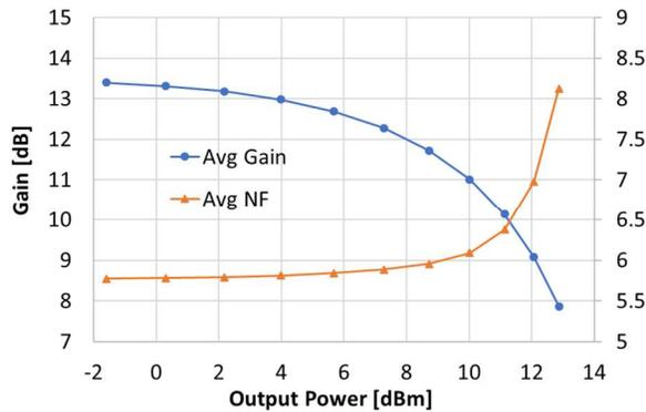
Fig. 3: Average gain and NF in 3.83 THz bandwidth
