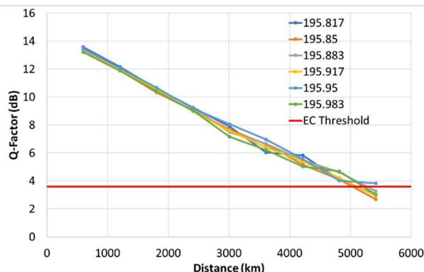
Fig 6: Performance vs. distance for six short wavelength channels
