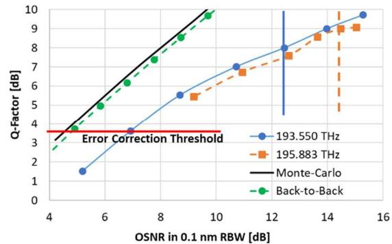
Fig. 4: Modulation format performance. Vertical lines indicate nominal OSNR for each channel
