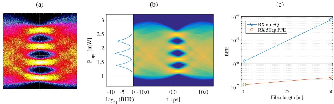
Fig. 3: 112 Gbit/s eye diagrams using (a) no RX EQ and (b) 5 RX taps, (c) BER using different lengths of fiber
