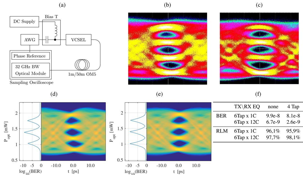
Fig. 2: (a) Experimental measurement setup, 80 Gbit/s eye diagrams using 6 TX taps of (b) linear FFE and (c) SC FFE, 80 Gbit/s eye diagrams with additional 4 taps linear FFE in the receiver using 6 TX taps of (d) linear FFE, (e) SC FFE, (f) overview of BER values
