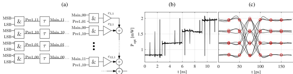
Fig. 1: (a) 1 Tap of Switched Coefficients FFE, (b) SC FFE training sequence, (c) overlaid pulse responses for all 12 combinations
