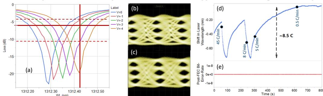
Fig. 4. (a) Transmission spectra resonance shift of MRM with applied bias, showing 6dB ER with 2V swing. Optical transmitted eye (b) without and (c) with pre-emphasis. (d) Laser wavelength shift during BER test, (e) post-FEC error rate over time.
