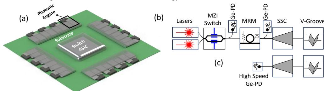
Fig. 1. (a) A 3-dimensional drawing of the integrated co-packaged optical IO switching system Schematic of 25.6 Tbps switch package with sixteen 1.6Tbps photonic engines. SiPIC architecture for each of 16 integrated Tx (b) and Rx (c) channels.
