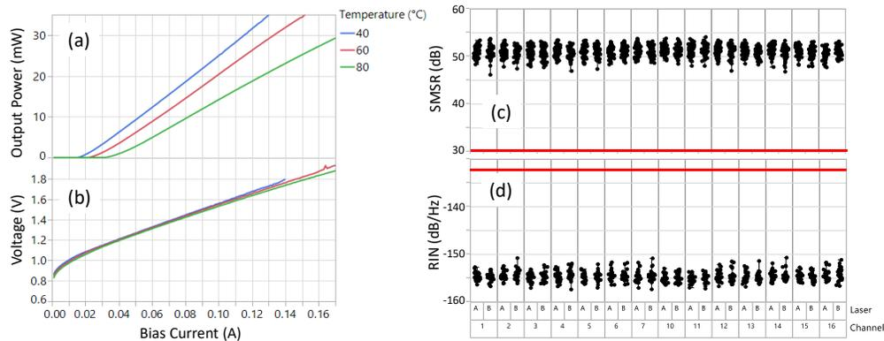
Fig. 2. (a) LI and (b) IV of an integrated hybrid III/V laser at 40, 60 and 80C. (c) SMSR at 25C and 130mA and (d) average RIN at 25C and 60mA for each of the 16 transmitter channels with redundant lasers A and B, across a 300mm wafer.
