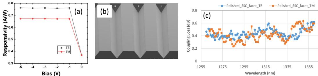
Fig. 3. (a) TE/TM mode Ge-PD Responsivity measured at room temperature, (b) Array of integrated V-grooves integrated with SiPIC, (c) Plot of actively aligned coupling loss to SMF fiber vs wavelength of two different coupler facets (optimized for TE and TM respectively).
