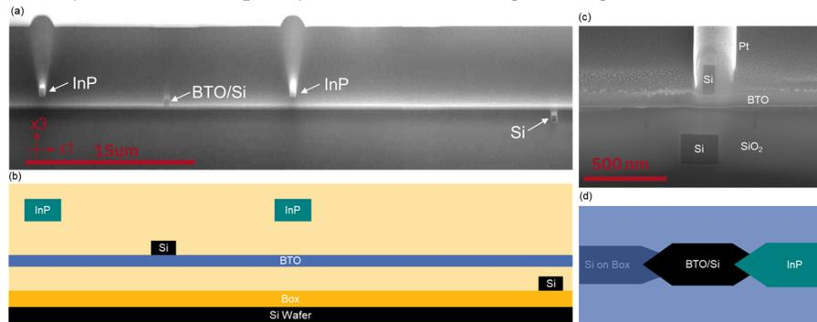
Fig. 2 (a) Focused Ion Beam (FIB) cross section showing two InP, a BTO/Si and a Si waveguide. (b) Schematic of the waveguides shown in the FIB cross section (a). (c) FIB cross section in coupler region (Si ↔ BTO/Si), showing a small offset in the lateral alignment. (d) Tapers are used to efficiently transfer guided light between the different layers.
