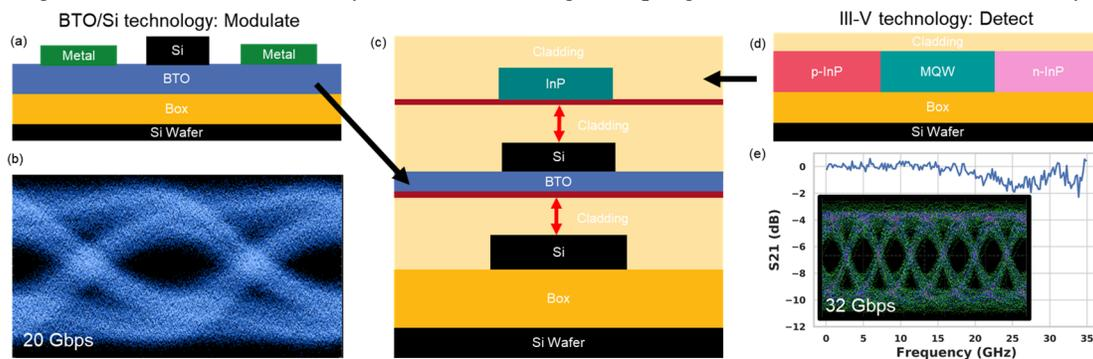
Fig. 1 (a) Schematic of Si/BTO modulator integrated on a Si wafer. (b) Eye diagram of a 20 Gbps signal from a Si/BTO modulator. (c) Schematic of demonstrator showing heterogeneous integration of Si, passive BTO/Si and passive III-V technology. (d) Schematic of a III-V detector, integrated on a Si wafer. (e) Frequency response of photodetector. Inset: Eye diagram at 32 Gbps (NRZ) without using digital signal processing.
