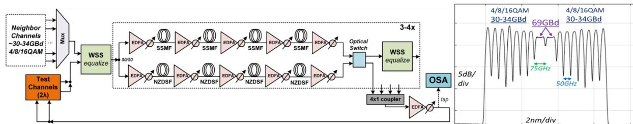
Fig. 1. Test-bed for SSMF and NZDSF transmission. Inset: OSA spectrum at transmit side (0.1 nm RBW) of the sixteen channel grid.
