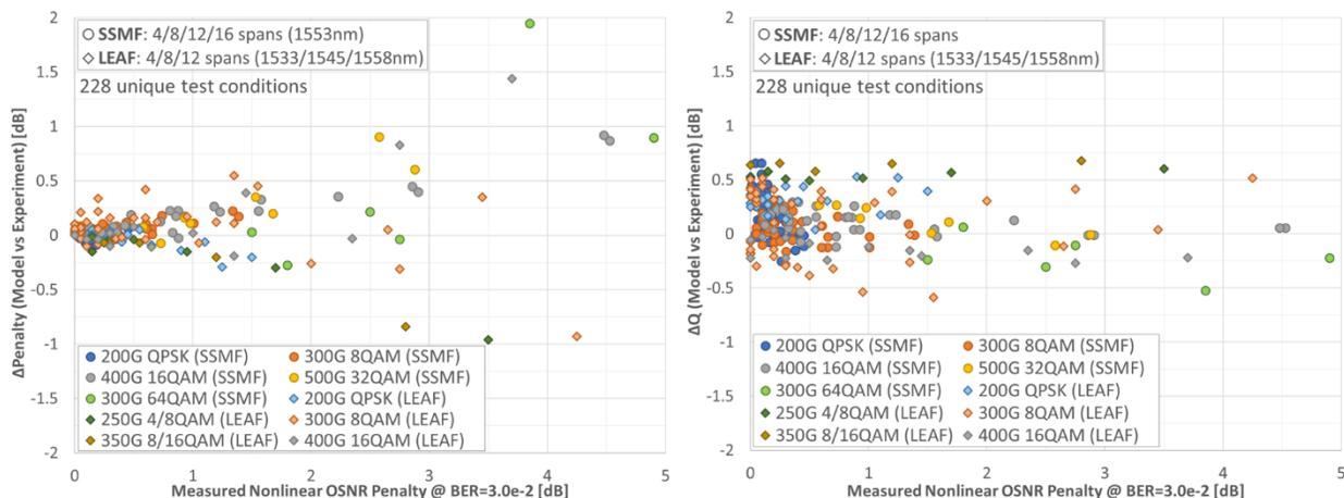
Fig. 4. Difference in (a) OSNR Penalty and (b) pre-FEC Q per channel between closed-form incoherent GN-model and experimental results, for all test data combined: SSMF and LEAF transmission, 69 GBd signals from QPSK up to 32QAM modulation and 34 GBd 64QAM signal.
