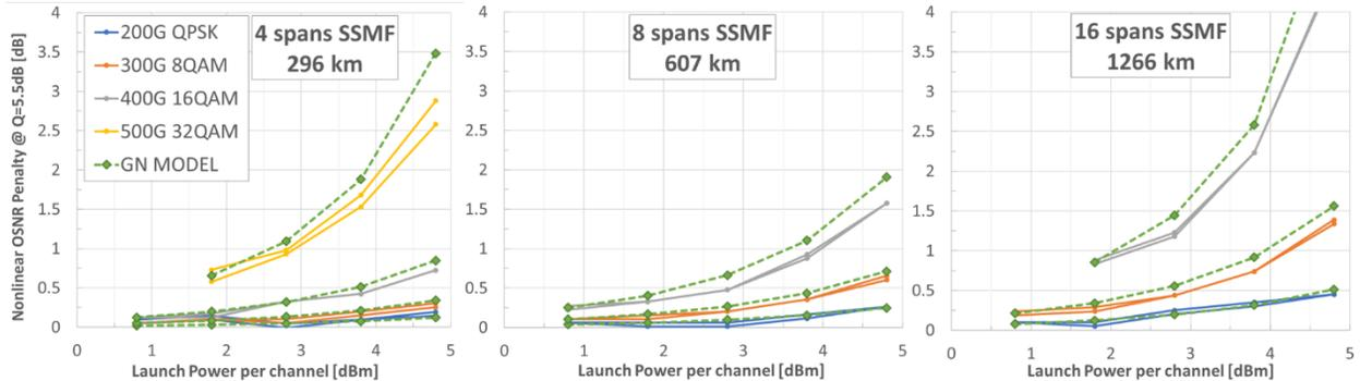
Fig. 2. Nonlinear OSNR penalty for 4, 8, and 16 spans SSMF. Both central test channels run at 69GBd and the same modulation format from the set: QPSK/8QAM/16QAM/32QAM; center  $\lambda = 1553$  nm. Green dashed lines: GN MODEL (closed-form incoherent) results.
