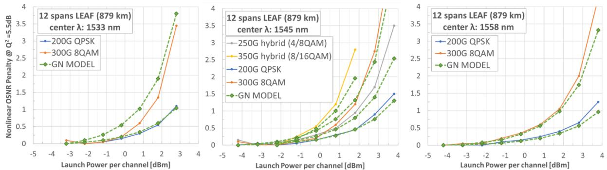
Fig. 3. Nonlinear OSNR penalty for 12 x 73km LEAF. Both central channels were run at 69 GBd and provisioned with different modulation formats. All cases used QPSK and 8QAM, and for 1545 nm case, hybrid modulation formats QPSK/8QAM and 8QAM/16QAM were also tested.
