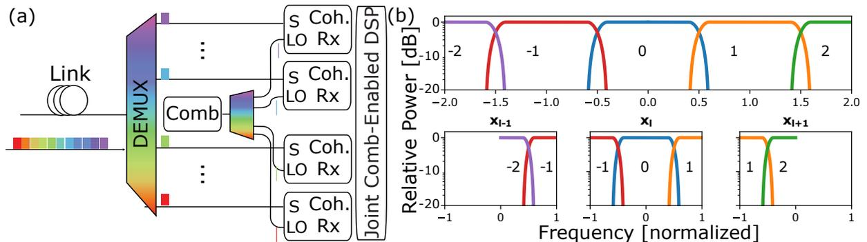
Fig. 1: (a) Principle sketch for a comb-based superchannel receiver. Each channel is detected using independent receivers with all LOs originating from a common frequency comb enabling joint DSP. (b) Frequency grid and inputs to the multi-channel equalizer using aliasing of the side channels to avoid upsampling. Each channel is sampled at 2SPS, or less, and stitched by the equalizer.
