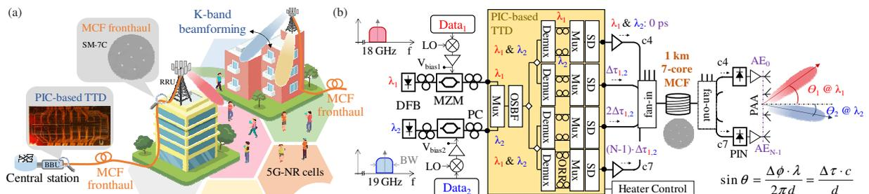
Fig. 1. (a) Multibeamformer application scenario in 5G-NR cells operating over MCF. (b) Experimental setup and block diagram of the dual-wavelength beamformer employing 1 km of 7-core MCF, providing independent tuning to each wavelength to steer the beam to  $\theta_1$  and  $\theta_2$
