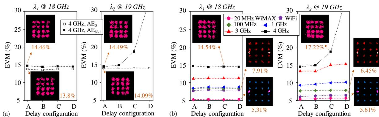
Fig. 3. (a) Measured EVM for 4-GHz BW signals comparing  $AE_0$  and  $AE_{N-1}$  performance in both wavelengths for different delay configurations corresponding to  $\Delta\tau_A \approx 0$  ps,  $\Delta\tau_B \approx 40$  ps,  $\Delta\tau_C \approx 260$  ps and  $\Delta\tau_D \approx 350$  ps. (b) Measured EVM for different delay configurations for  $AE_{N-1}$  in both wavelengths. Example of received 16QAM constellations and EVM values included as insets.
