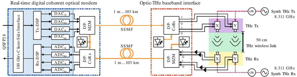
Fig. 1. Experimental setup depicting the optic-THz baseband interface that translates the polarization-multiplexed optical signal into the electrical domain, so that data can be transmitted over a THz wireless link, which operates at a carrier frequency of  $\sim 300$  GHz.
