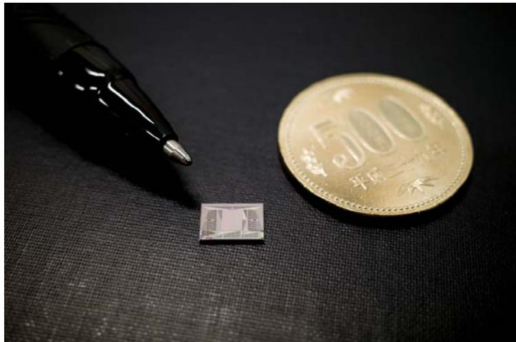
Fig. 1 Si photonics FMCW LiDAR chip equipped with nonmechanical beam steering device, modulator and PDs.
