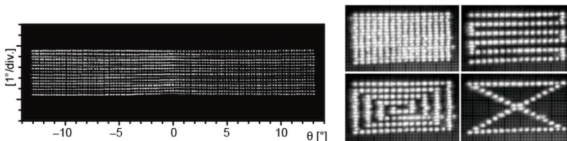
Fig. 2 Wide 2D beam steering (left) and flexible steering (right).
