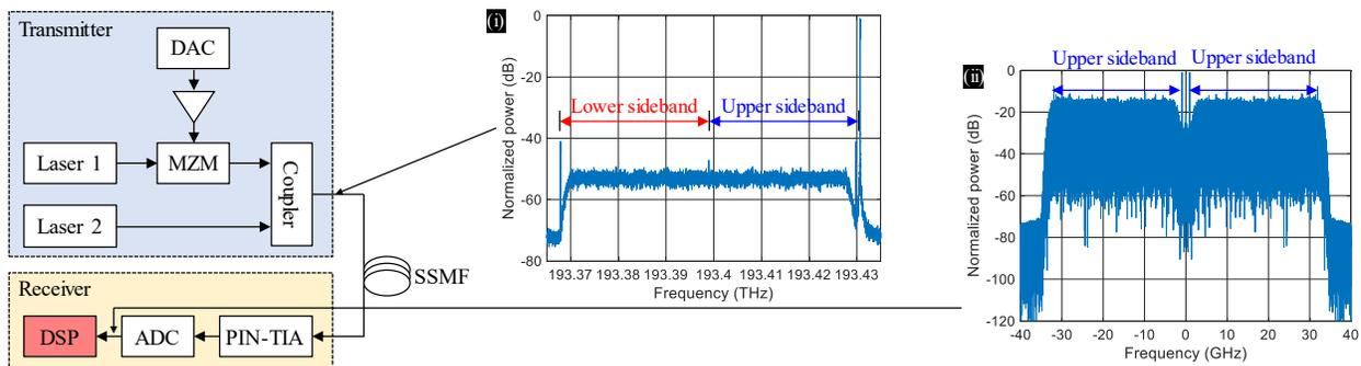
Fig. 2. Experimental setup used to evaluate the proposed scheme. (i) Optical spectrum measured at the output of the transmitter. (ii) Photocurrent spectrum at the receiver.
