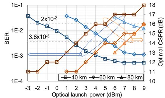
Fig. 4. Optimal CSPP and corresponding performance after SSBI mitigation measured at various optical launch powers for 40 km, 60 km and 80 km transmission.
