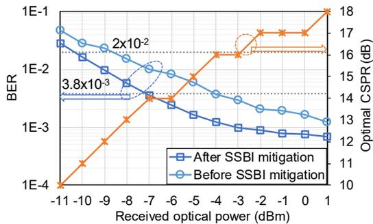
Fig. 3. Optimal CSPP and corresponding performance measured at various received optical powers in back-to-back configuration.
