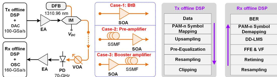
Fig.1. Experimental setup and three different transmission cases with detailed Tx and Rx offline DSP blocks.
