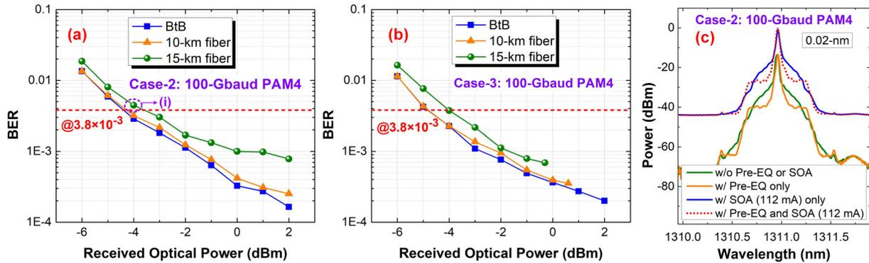
Fig. 3. Experimental results for 100Gbaud PAM4. (a) and (b) BER versus ROP under case-2 and case-3, respectively; (c) the optical spectra of 100 Gbaud PAM4 signal with different cases.
