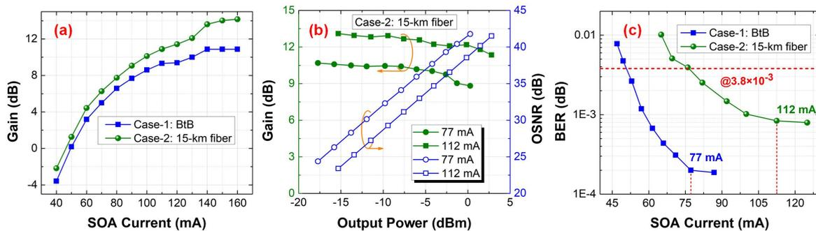
Fig.2. The performance of SOA for 100 Gbaud PAM4 signal. (a) SOA gain versus SOA bias current; (b) SOA gain and OSNR versus output power; (c) BER versus SOA bias current.
