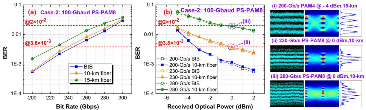
Fig. 4. Experimental results for 100 Gbaud PS-PAM8. (a) and (b) BER versus different bit rates and ROP under case-2, respectively. Insets (i)-(iii) are recovered symbols, eye diagrams and histograms, respectively.
