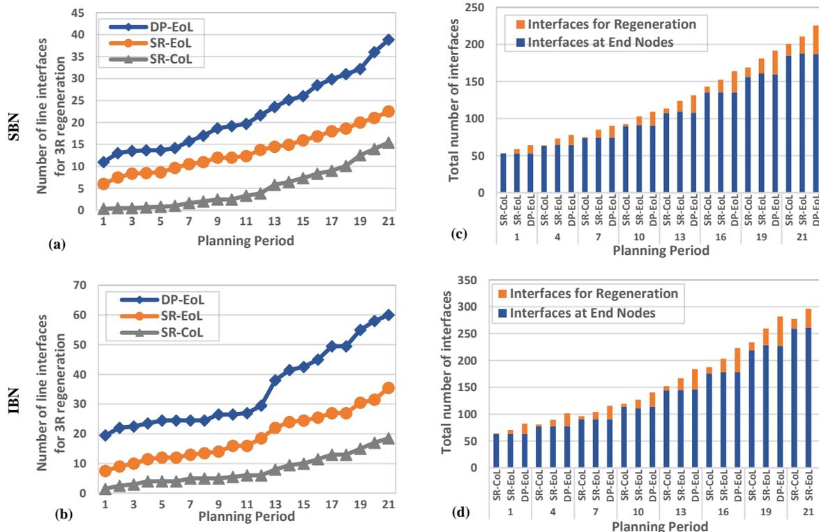
Fig. 2. (a-b) Evolution of the number of line interfaces that have to be deployed for regeneration in the backup paths and (c-d) evolution of the total number of line interfaces that have to be acquired throughout network operation for both network topologies.
