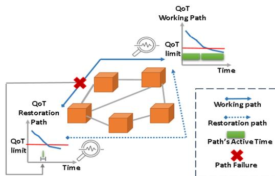
Fig. 1. Optical restoration with reduced performance margins.
