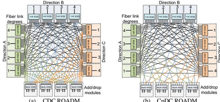
Fig. 1. Comparison between CDC and CpDC ROADMs architectures.
