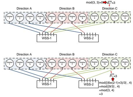
Fig. 2. Example of the interconnection pattern.
