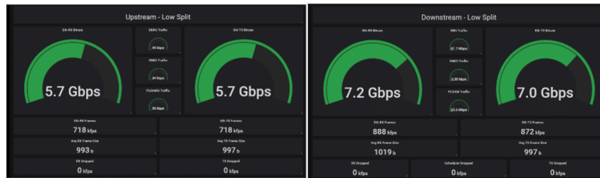
Fig. 3. Upstream and Downstream throughput (Gbps) for fully softwareised OLT
