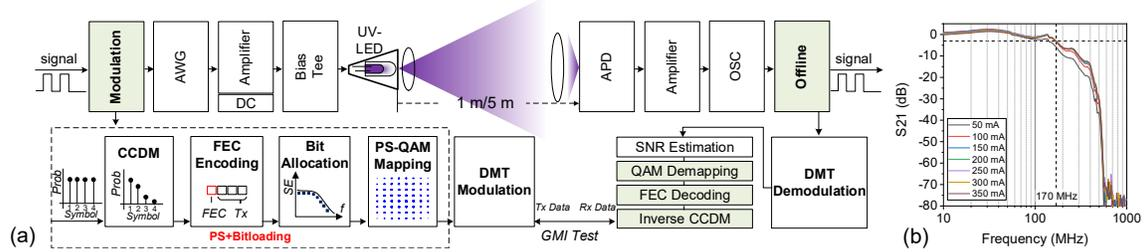
Fig. 1: (a) The experimental setup and the flow diagram of the signal generation and offline processing. (b) The modulation bandwidth of the system at a distance of 5 m with different injection currents.
