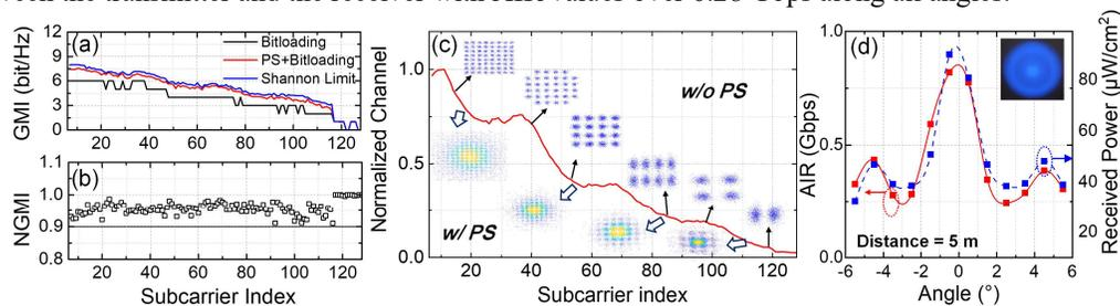
Fig. 3: (a) The GMI for the different subcarriers before and after using PS at a distance of 5 m. (b) The NGMI of the different subcarriers. (c) The constellation diagrams of the received signal with and without PS. (d) The GMI and the received power per unit area of the 5-m diffuse-LOS link at different angles, and the inset is a picture of the beam profile. The 11% FEC overhead was removed in the AIR calculation.
