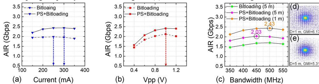
Fig. 2: The AIR at different (a) injection currents, (b) signal amplitudes, and (c) signal bandwidths. The PS constellation diagram at transmission distances of (d) 1 m and (e) 5 m. All AIR values are calculated after removing the 11% FEC overhead.
