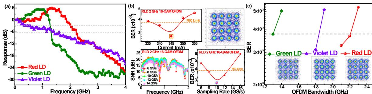
Fig. 3. (a) Analog modulation responses of the red LD, green LD and violet LD with each optimized bias current. (b) BER versus bias current, constellation plot, and SNR spectra and BER under different sampling rates for 16-QAM OFDM data carried by R-LD. (c) Bandwidth dependent BERs of the 16-QAM OFDM data carried by R/G/V LDs before and after pre-leveling optimization.
