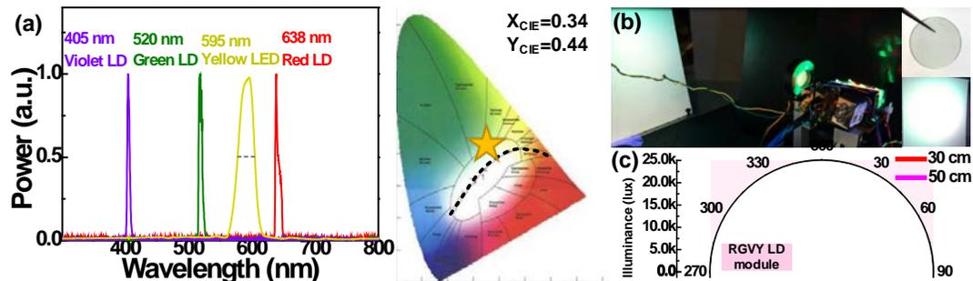
Fig. 2. (a) Optical and CIE spectra of the R/G/V LDs and yellow LED. (b) The photographs of the miniature R/G/V/Y mixed white-lighting module and its lighting spot on white paper. (c) The angle-dependent illuminance distribution of the R/G/V/Y mixed white-light module.
