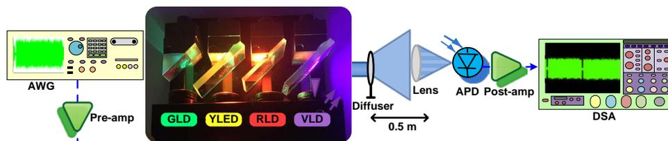
Fig. 1. The photograph of the miniature R/G/V/Y module and the experimental setup for white-lighting communication.
