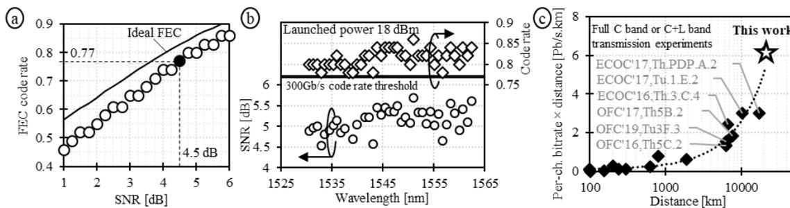
Fig. 2: a) Back-to-back characterization of FEC decoder family, b) measured SNR and maximum code rate of the 41 C-band channels after 20570 km, and c) evolution of per-channel bit rate times distance product in transoceanic capacity record experiments
