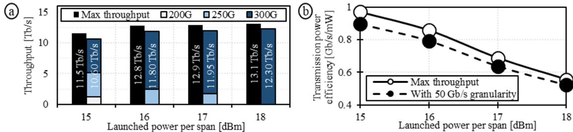
Fig. 3: a) maximum achievable throughput and b) transmission power efficiency versus launched power per span after 20570 km
