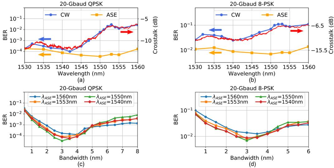
**Fig. 3:** Measured BER as a function of source central wavelength of (a) QPSK and (b) 8-PSK signal for both conventional coherent detection and low-coherence matched detection with  $B_{\text{ase}}=3$  nm, BER versus  $B_{\text{ase}}$  of (c) QPSK and (d) 8-PSK signal at different central wavelengths.
