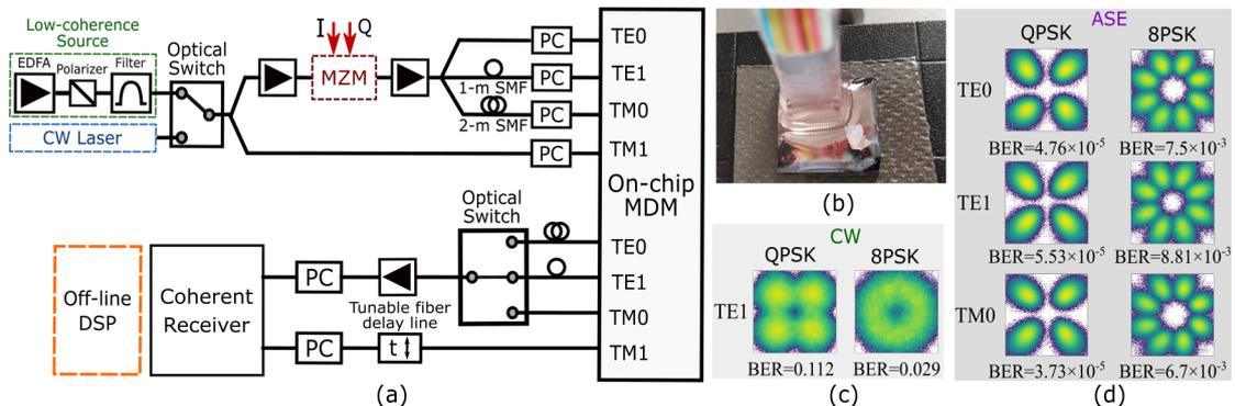
**Fig. 2:** (a) Setup for on-chip MDM transmission with modal crosstalk mitigation employing low-coherence matched detection, (b) photo of the fully packaged MDM circuit, BER and constellation of QPSK and 8-PSK signals using (c) conventional coherence detection using CW light for the  $TE_1$  mode and (d) low-coherence matched detection with  $B_{ase}=3$  nm for the three modes.
