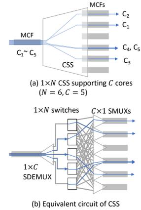
Fig. 4. CSS functionality and its equivalent circuit.
