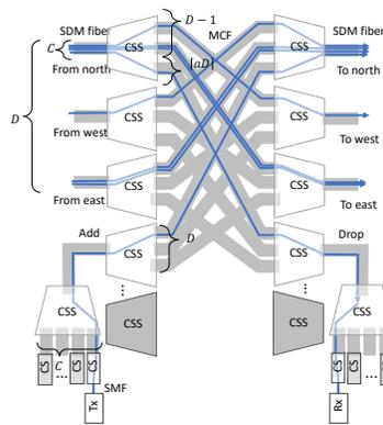
Fig. 5. CSS-based SXC architecture (*any-core access and non-directional with core-contention*).
