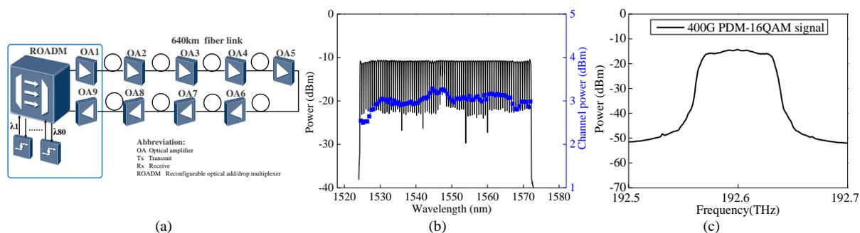
Fig. 1: (a) Experimental set up for the 32Tb/s transmission; (b) Measured spectrum over the 48nm super C band and optical power per channel at the output of the fifth optical amplifier; (c) Measured optical spectrum for the 400-Gb/s PDM-16QAM signal.
