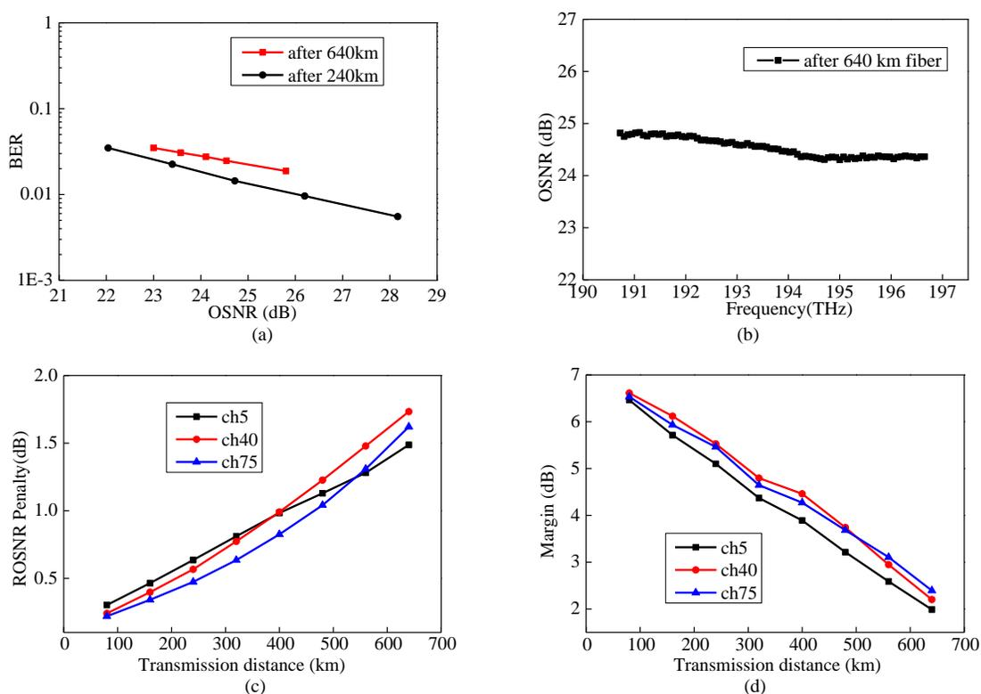
Fig. 2: (a) BER versus OSNR for transmissions over 240km and 640km distance; (b) Measured OSNR spectrum over the 48nm super C bandwidth; (c) Measured required OSNR (ROSNR) penalty versus transmission distance for selected channels; (d) Measured OSNR margin vs transmission length for selected channels.
