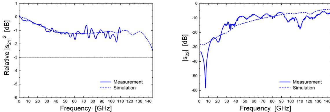
Fig. 3. RF transmission response (left) and electrical reflection (right) for a reverse bias voltage of  $2\text{V}$
