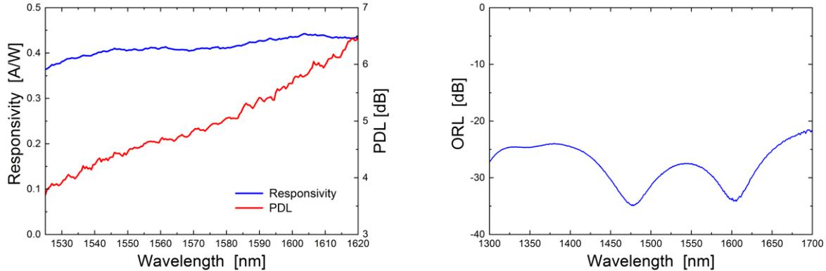
Fig. 2. Responsivity and polarisation dependent loss measurement (left) and optical return loss measurement (right)
