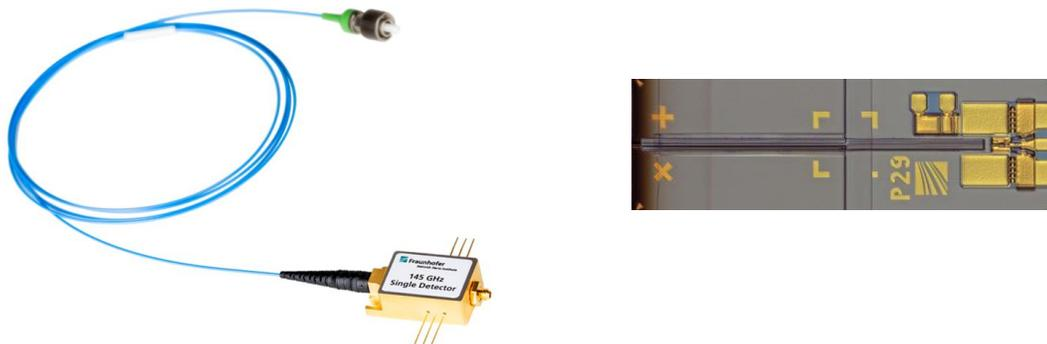
Fig. 1. Fabricated high-speed photodetector module (left) and top view of the photodetector chip inside the module (right)
