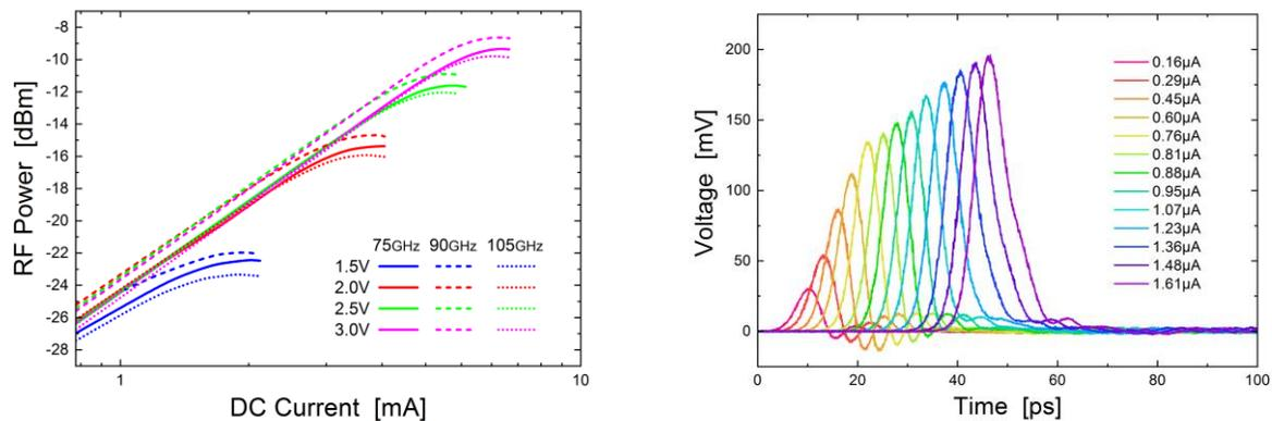
Fig. 4. Linearity measurements for different reverse bias voltages and perturbation frequencies (left) and pulse response for different optical input powers at a reverse bias voltage of 2V (right); legend of pulse response measurement indicates measured average DC-bias current at the photodetector module for different power of the pulses
