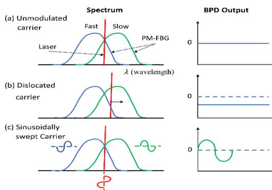
Fig 1: Operating principle of the proposed scheme: The reflection spectrum of PM-FBG relative to laser (left) and the corresponding output of BPD (right) for (a) unmodulated carrier, (b) dislocated carrier, and (c) sinusoidally swept carrier cases.
