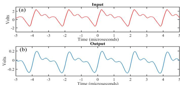
Fig 4. (a) Input to the EOM for modulating an optical carrier tuned at the crossover wavelength of PM-FBG. (b) Output of the BPD.
