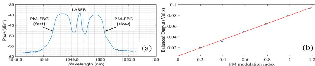
Fig 3: (a) Laser wavelength is tuned to the crossover point between the two PM-FBG Bragg peaks. The spectrum is measured by simultaneously coupling outputs from a mode-locked laser and the DL into the PM-FBG. (b) Measurements of peak-to-peak voltage at output of BPD as FM modulation index is increased (blue cross marks). Red line represents linear fitting.
