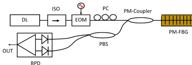
Fig 2: Schematic of the experimental setup for FM demodulation. DL: diode laser, ISO: fiber-coupled isolator, EOM: electro-optic modulator, PBS: polarization beam splitter, PC: polarization controller, PM-Coupler: polarization-maintaining coupler.
