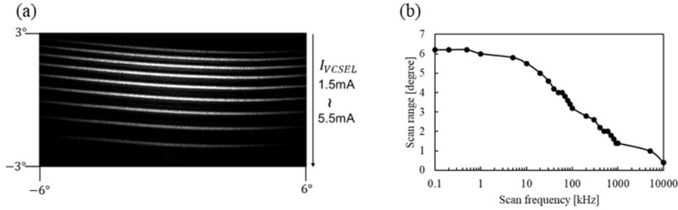
Fig. 2 (a) Reflected pattern (b) Scan frequency and range of the beam scanner.
