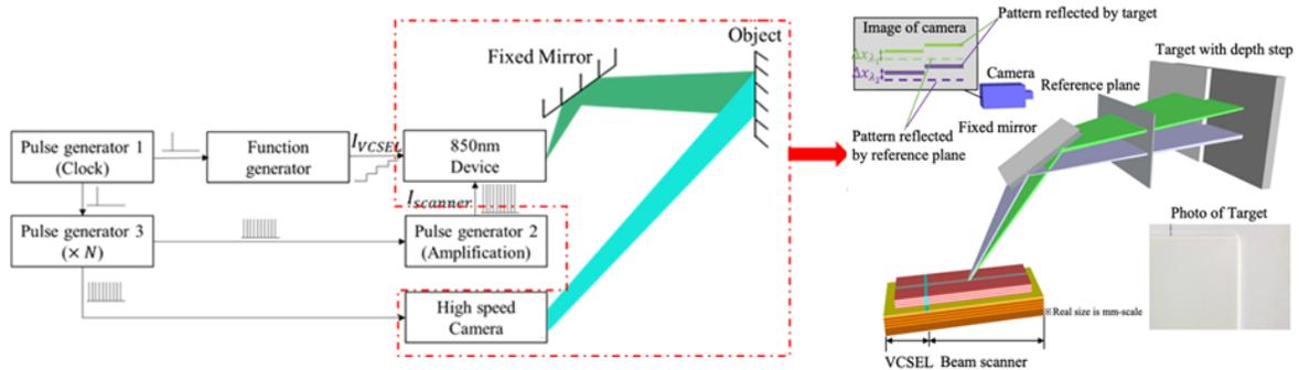
Fig. 3 Schematic of synchronization system and structured-light depth sensing system
