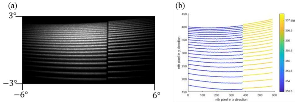
Fig. 4 (a) Pattern reflected by the target (b) single depth image of the target.
