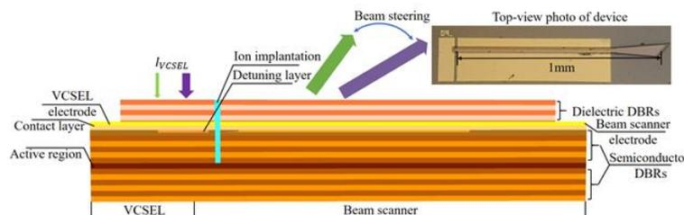
Fig. 1 The structure of beam scanner integrated to a tunable seed VCSEL.
