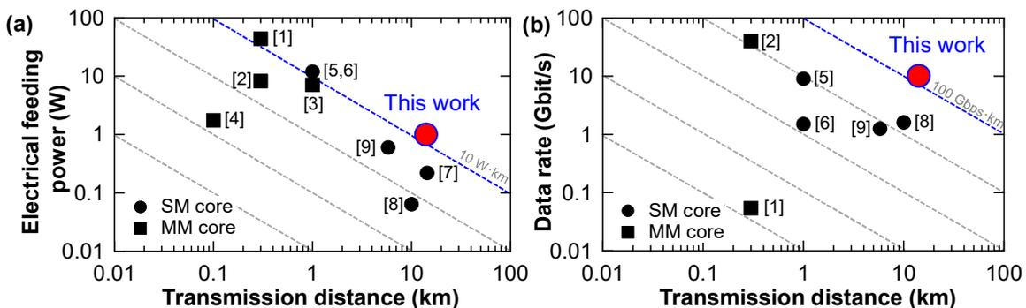
**Fig. 1** Relationship between (a) electrical feeding power and transmission distance and (b) data rate and transmission distance in various PoF experiments.
