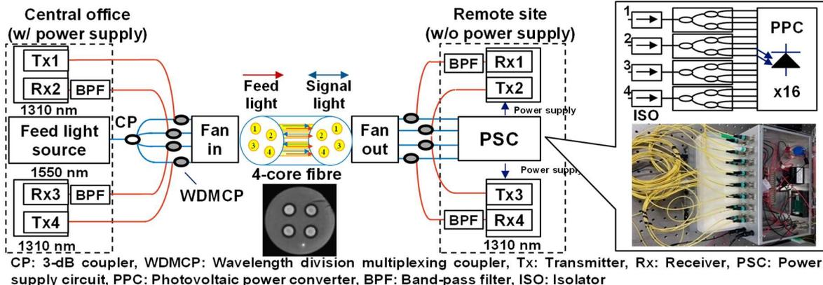
Fig. 2 Schematic diagram of PoF system using 4-core fibre and configuration of power supply circuit (PSC).
