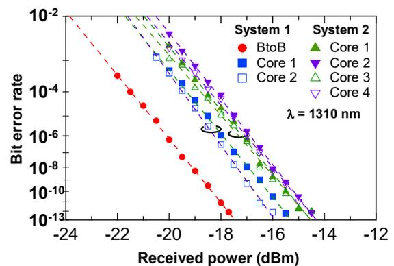
**Fig. 4** Measured BER performance of 14.1-km-long one-pair and 6.0-km-long two-pair bi-directional data links as a function of received power.
