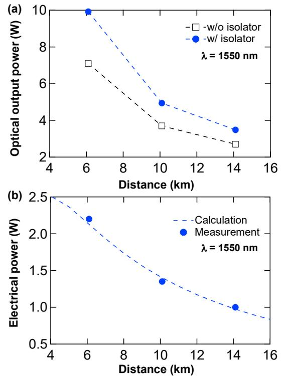
**Fig. 3** (a) Relationship between optical output power and distance of 4-core fibre with and without isolators. (b) Calculation and measurement results of electrical power vs. transmission distance for PoF system.
