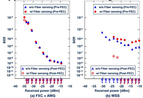
Fig. 5: BER characteristics of 100-Gbit/s DWDM signal.
