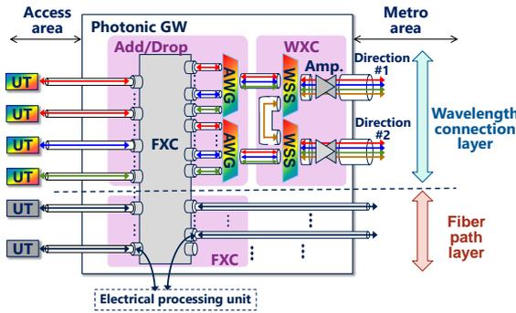
Fig. 2: Example configuration of Photonic GW.
