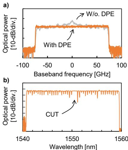
**Fig. 3.** Optical spectrum of a) the channel under test (CUT) at the transmitter output; b) the WDM channel comb after 1 loop (605-km).
