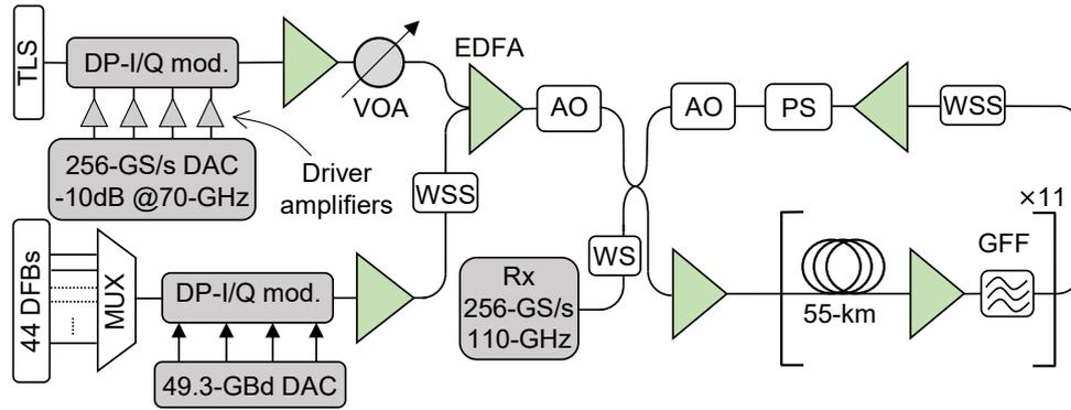
**Fig. 2.** a) Experimental setup. WSS: wavelength selective switch; WS: Wave Shaper; PS: polarization scrambler; AO: acousto-optics switch. VOA: Variable Optical Attenuator. EDFA: Erbium doped fiber amplifier. GFF: Gain flattening filter.
