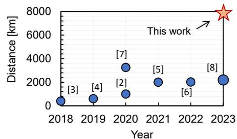
Fig. 1. Achieved transmission reaches for 800-Gbps per wavelength transmissions.
