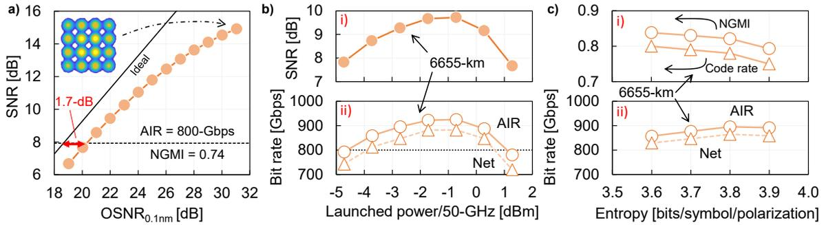
**Fig. 4.** Experimental results. a) Back-to-back sensitivity to noise of the 148-GBaud DP-PCS-16QAM signal. b) SNR and bit rate versus launched power. c) Entropy optimization : code rate, NGMI and bit rate at the optimum launched power.
