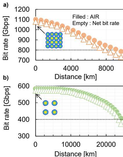
**Fig. 5.** Bit rate versus transmission distance. a) DP-PCS-16QAM at 148-GBaud. b) DP-QPSK.
