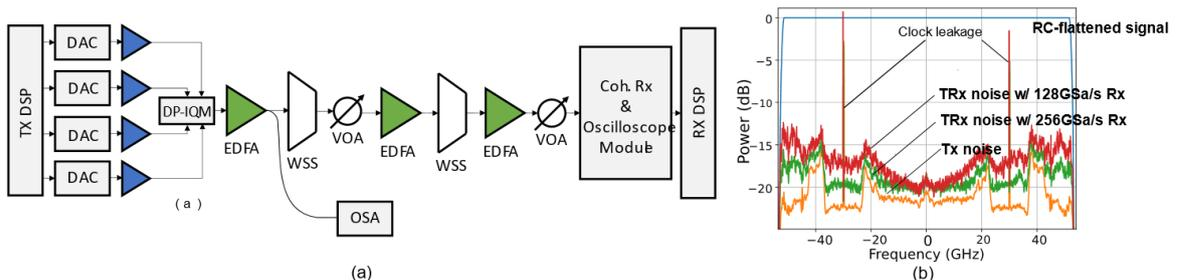
Figure 2 (a) Experimental Setup (b) raised-cosine flattened signal and noises
