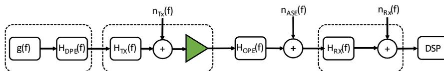
Figure 1 Simplified System Model
