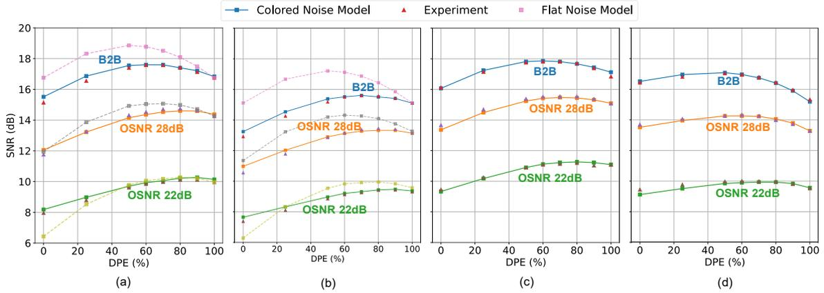
**Figure 3** Model prediction of SNR vs DPE at 105 Gbaud (a) 256GSa/s ADC (b) 128GSa/s ADC (c) 256GSa/s ADC with 30% OPE (d) SCM with 8 subcarriers (global SNR is used as a metric [13])
