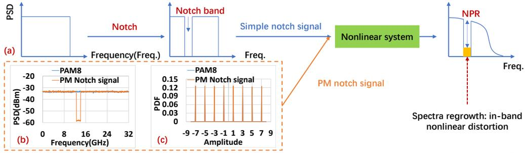
Fig. 1: (a) Schematic of the conventional NPR method, (b) the spectrum and (c) the PDF of a PM notch signal. PSD: power spectrum density
