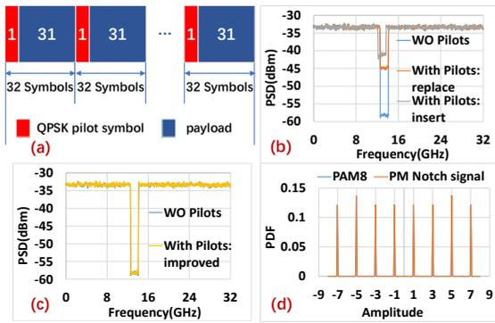
Fig. 2: (a) The frame structure used in this study, the spectrum of the PM notch signal with pilot symbols realized by the (b) straightforward methods and (c) improved method, and (d) the PDF of the PM notch signal and normal communication signal with QPSK pilot symbols.
