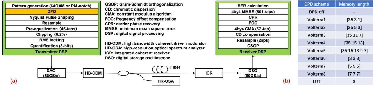
Fig. 4: (a) Experimental setup of the unamplified system with 10-km transmission and (b) the memory length and order of different DPD schemes.
