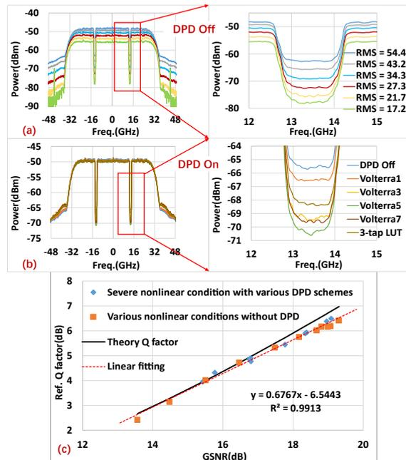
Fig. 5: Spectra measured by the PM NPR method for (a) various nonlinear conditions without DPD and (b) severe nonlinear condition with various DPD schemes, (c) the reference Q factor and theory Q factor versus the measured mean GSNR
