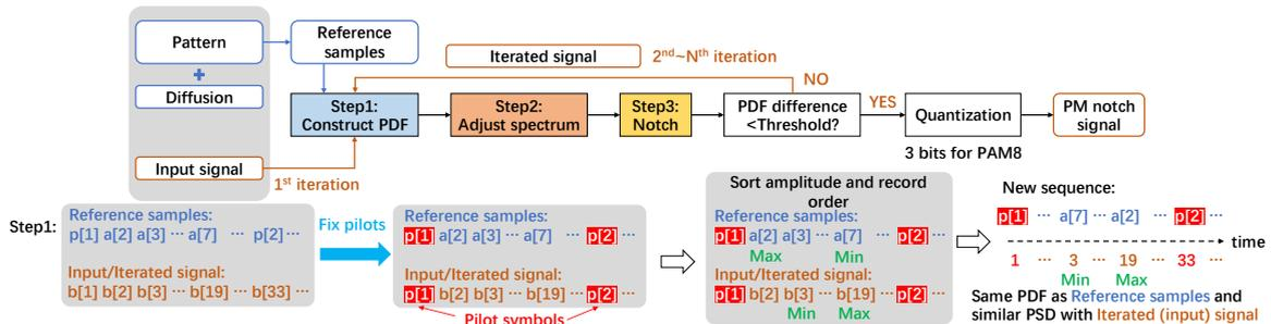
Fig. 3: Principle of the improved search method for PM notch signals with pre-defined pilot symbols.
