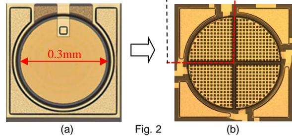
Fig. 1 (a) Cross-sectional view of a two-stacked PIN-PD block, (b) schematic circuit diagram of four series connected two-stacked PIN-PD blocks, Fig. 2(a) top-view of 0.3 mm diameter conventional PIN-PD, (b) fabricated 0.3 mm diameter four-series connected two-stacked PIN-PD blocks
