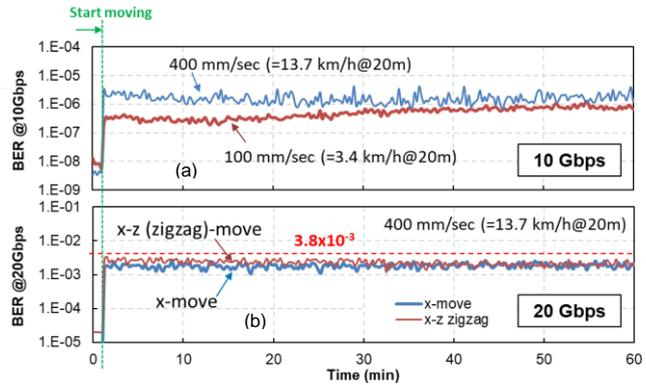
Fig. 7 (a) 10 Gbps BER variation in 1 hour when moving the stage at moving speed of 100 and 400 mm/sec, (b) 20 Gbps BER variation with simultaneous moving to x-z direction (zigzag) and only to x direction at 400 mm/sec
