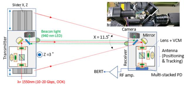
Fig. 4 Experimental setup for movable FSO communication demonstration at 400 mm/sec in 2.1 m
