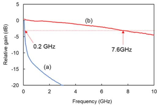
Fig. 3 Frequency response for (a) conventional  $\Phi$ 0.3 mm PIN-PD, (b) fabricated two-stacked  $\Phi$ 0.3 mm PIN-PD
