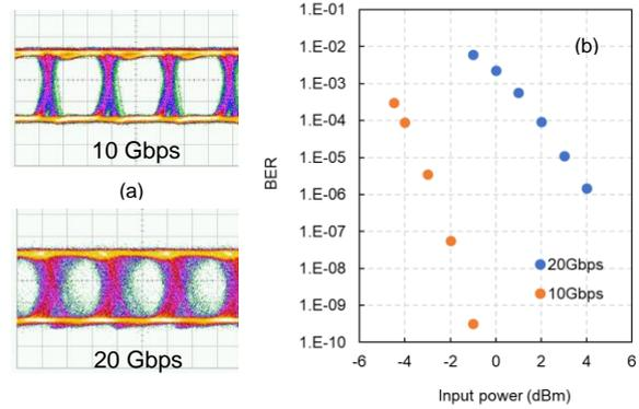
Fig. 6(a)(b) Eye diagrams and BER curves at 10/20 Gbps (OOK) when the stage is stopped,
