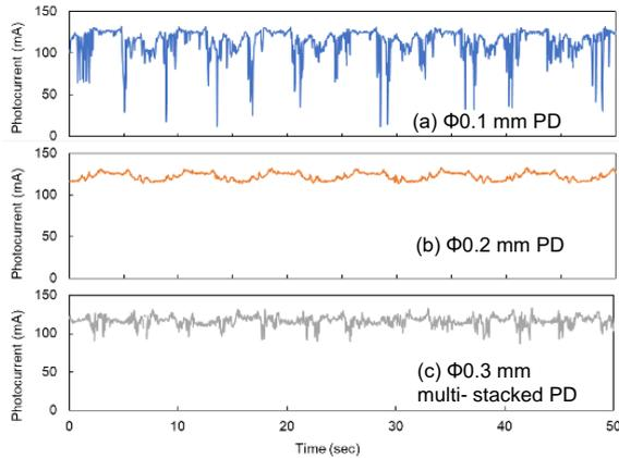
Fig. 5 Tracking and alignment testing in the FSO system while moving stage using (a) (b) 0.1-mm and 0.2-mm diameter conventional PDs, (c) newly developed two-stacked 0.3mm PD
