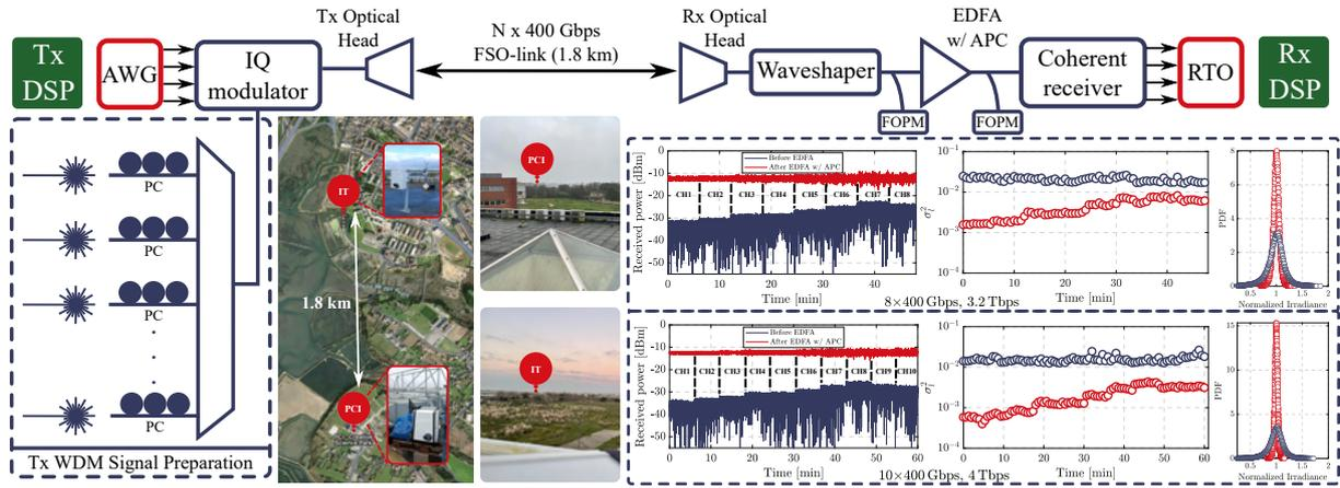
**Fig. 1:** Field trial of multi-terabit WDM coherent transmission over a 1.8 km FSO link between IT-Aveiro and PCI-Ilhavo, depicted with a Google Maps top-view highlighting the communications terminals. Channel-wise received optical power and turbulence strength are also depicted for 8 and 10 wavelengths.
