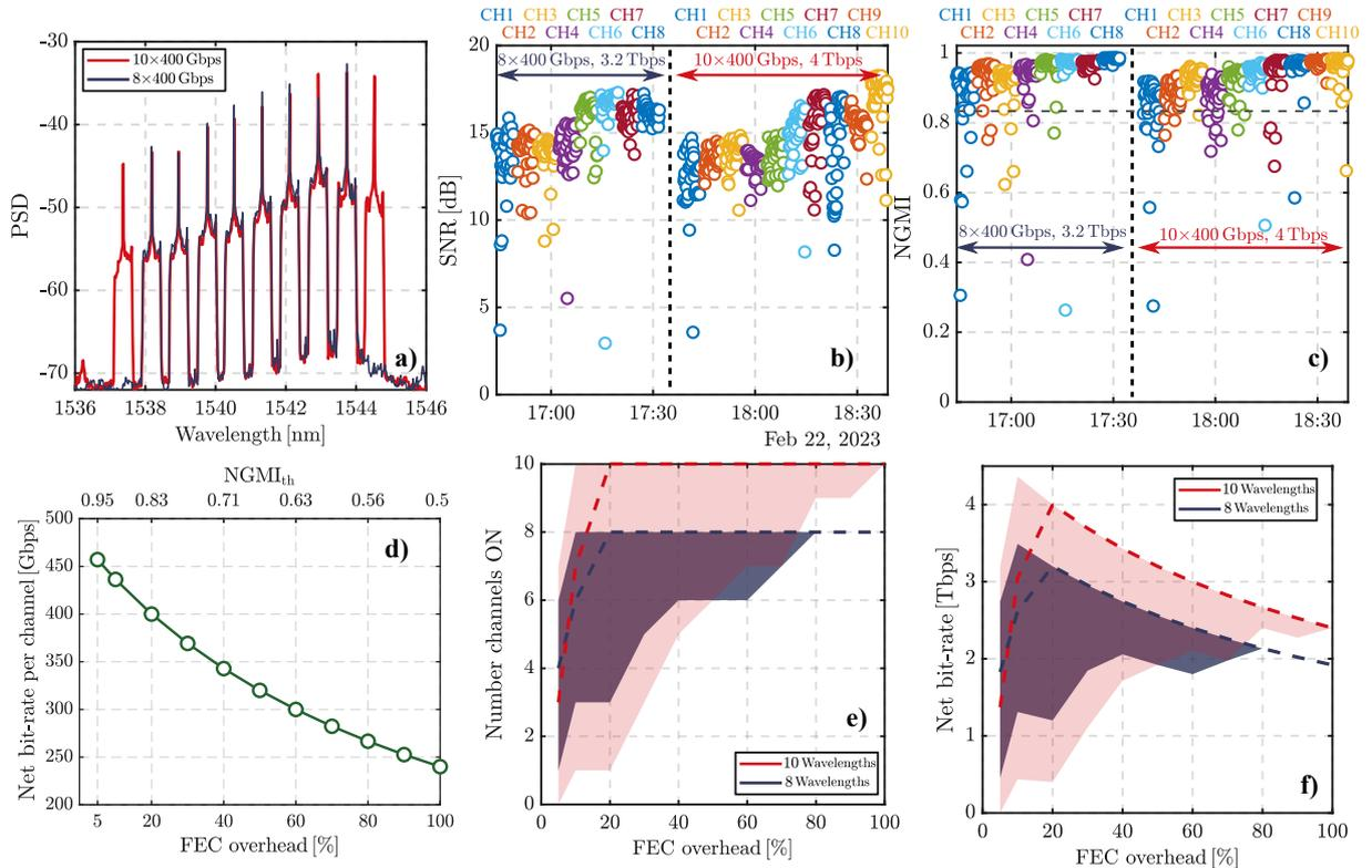
**Fig. 2:** Results obtained from multi-terabit WDM transmission over a 1.8 km FSO-link: a) received optical spectrum before filtering with 8 and 10 wavelengths; b) measured electrical SNR per channel; c) measured NGMI per channel; d) impact of FEC overhead in the net bit-rate per channel; e) evolution of the number of supported wavelengths versus the FEC overhead; and f) minimum, maximum, and average net capacity obtained by changing the FEC overhead.
