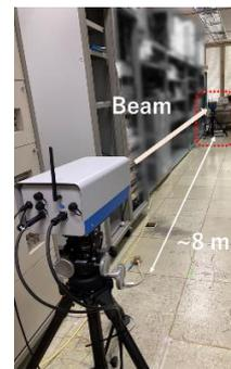
Fig. 1: Picture of all-optical FSO transceivers for a FSO-CL.
