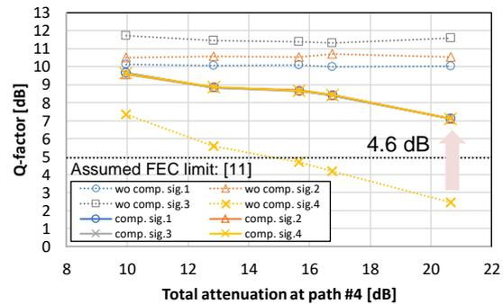
Fig. 4: Experimental results of attenuation dependency with all-optical FSO transceivers for a FSO-CL #4.
