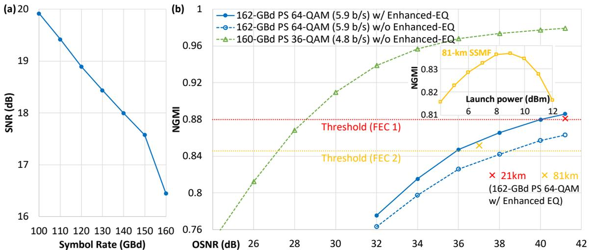
**Fig. 3:** (a) System B2B SNR as a function of symbol rate (evaluated by uniform 64-QAM signals); (b) OSNR sensitivity for the two formats as summarized in Fig. 2(i); (b-inset) NGMI of the PS 64-QAM signal as a function of fiber launch power (81-km SSMF).
