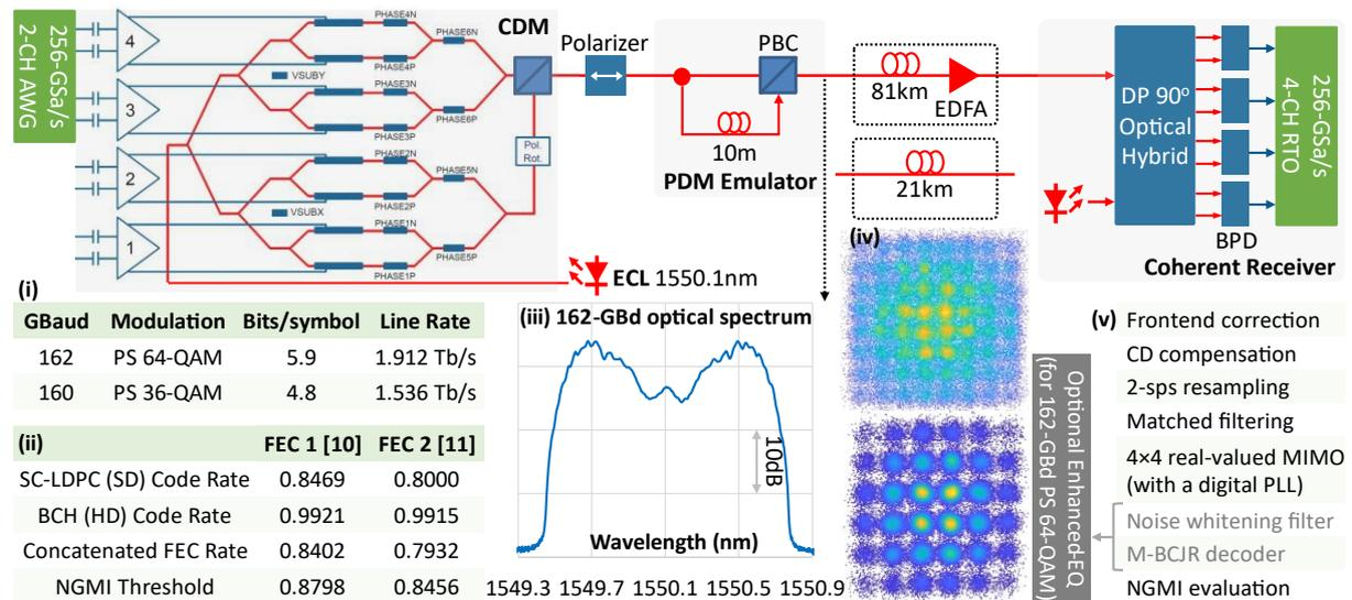
**Fig. 2:** Experimental setup. Inset (i) modulation formats evaluated in the experiment; (ii) two concatenated FEC schemes [11, 12]; (iii) transmitter output spectrum; (iv) (back-to-back) received PS 64/36-QAM constellations at the maximum OSNR of 41.2 dB; (v) receiver offline DSP. PBC: polarization beam combiner; PDM: polarization division multiplexing; PLL: phase locked loop.
