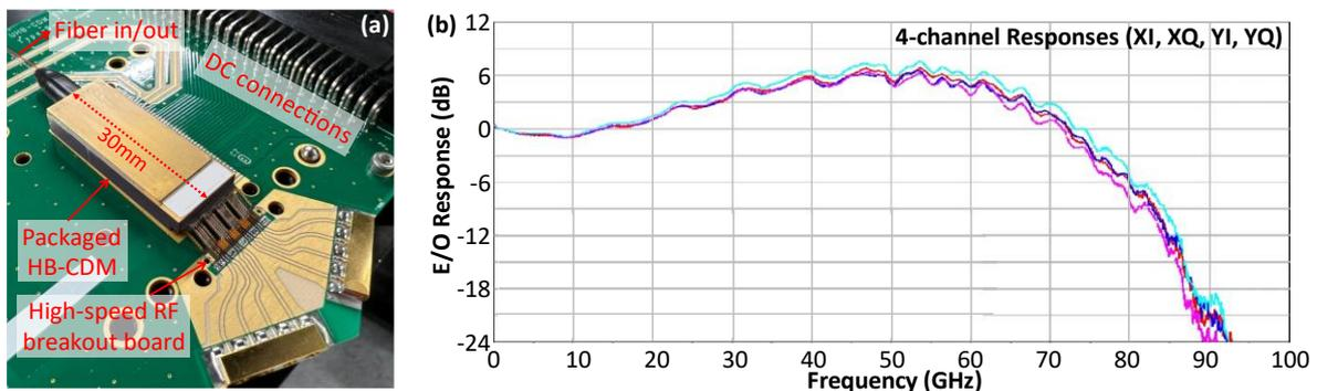
Fig. 1: (a) The fully packaged CDM mounted on an EVB; (b) E/O response of the entire module (at 1550 nm, room temperature).
