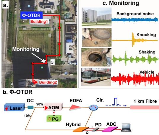
**Fig. 1:** (a) A field experiment using  $\Phi$ -OTDR; (b) The  $\Phi$ -OTDR system based on the I/Q demodulator. OC: optical coupler, AOM: acoustic optic modulator, EDFA: erbium-doped fiber amplifier, Cir.: circulator, PG: pulse generator, PD: photodetector, ADC: analog-to-digital converter; (c) Monitoring of four types of events.
