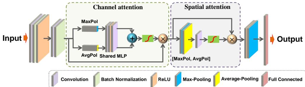
**Fig. 2:** The network structure of CS-CNN.
