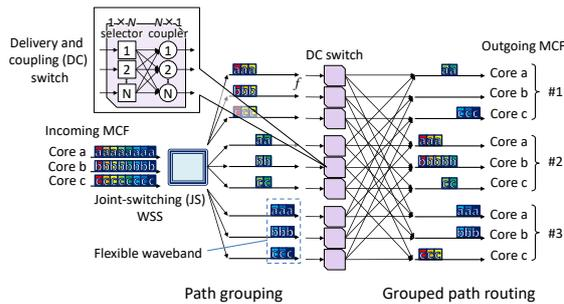
Fig. 3: Spatially-joint path grouping and routing.
