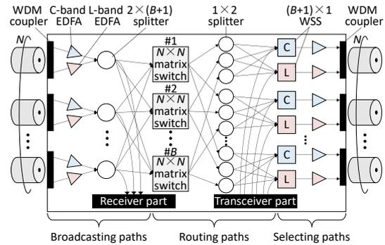
Fig. 4: Flexible Waveband Routing Node for Multi-band Networks [21].
