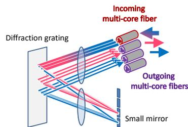
Fig. 2: Spatially-joint switching at a MEMS-based WSS.
