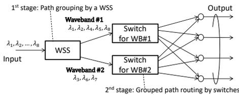
Fig. 1: Two-stage routing scheme.
