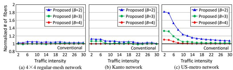
Fig. 6: The normalized number of necessary fibres relative to WSS-based node [21].
