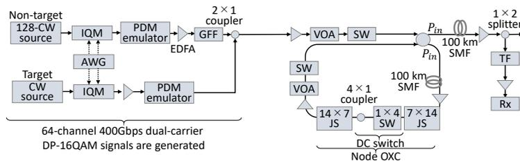
Fig. 7: Experimental configuration [20].
