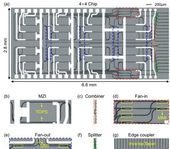
**Fig. 1:** Micrographs of (a) the  $4 \times 4$  SiN integrated chip. (b) A Mach-Zehnder Interferometer (MZI) unit equipped with two thermo-optic phase shifters (TOPSs). (c) a Combiner block. (d) a Fan-in block consisting of cascaded multi-mode interferometers (MMIs). (e) a Fan-out block consisting of MMIs. (f) a Splitter block. (g) Edge couplers with the inverse taper structure.
