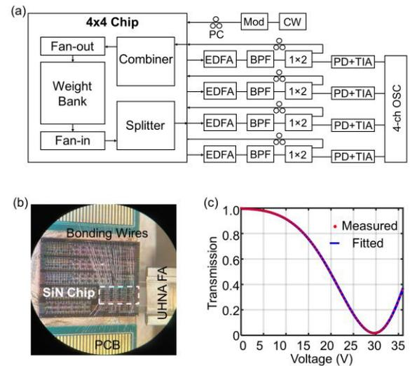
**Fig. 2:** (a) Experimental setup of the all-optical iterative matrix inverter. (b) Packaged chip. (c) Calibrated exemplary MZI transmission curve
