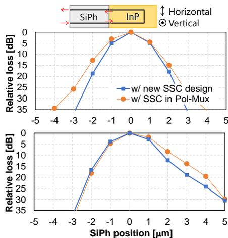
Fig. 5: InP-SiPh tolerance curve (a) horizontal and (b) vertical.
