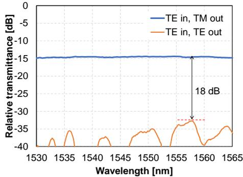
Fig. 3: Relative transmittance via TE-TM rotator and PBC.
