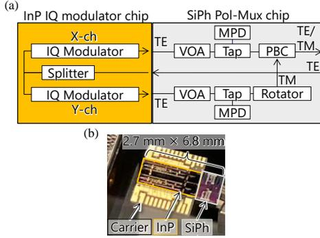
Fig. 2: (a) Block diagram and (b) photograph of fabricated DP-IQ modulator.
