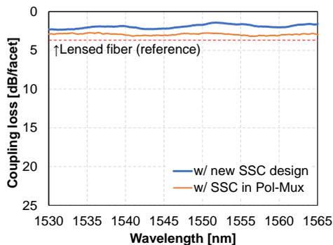
Fig. 6: InP-SiPh coupling loss.
