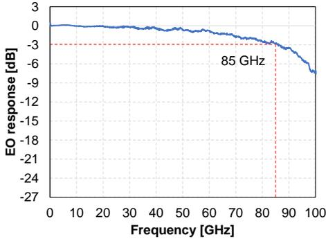
Fig. 4: Small signal EO response.
