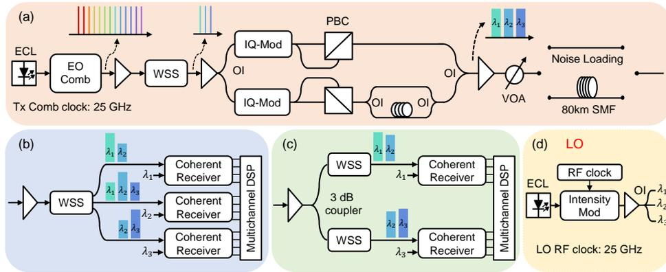
**Fig. 2:** Experimental setup. (a) Transmitter and channel, (b) Three receivers diagram, (c) Two receivers diagram, (d) LO setting.
