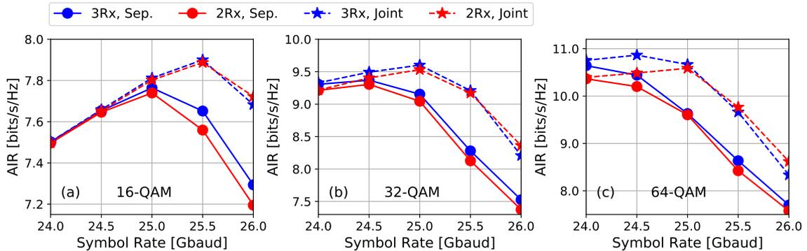
**Fig. 4:** Achievable information rate of the center channel versus symbol rate after 80-km SMF. The proposed two-receivers diagram (2Rx, performed following Fig.1 (b)) is compared with the three-receivers diagram (3Rx, performed following Fig.1 (a)) in terms of separate and joint processing.
