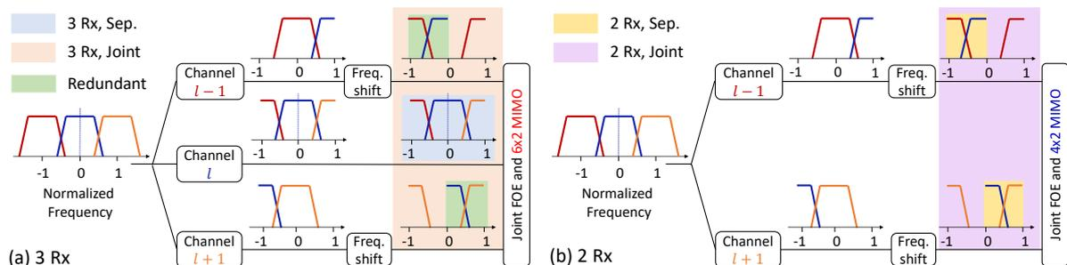
**Fig. 1:** Multi-channel processing enabled by (a) Three receivers, (b) Two receivers. The green bars in (a) highlight the redundant detection of the center channel  $l$ . The processing operates at 2 SPS. Sep.: separate processing; Joint: joint processing.
