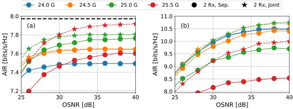
**Fig. 3:** Achievable information rate of the center channel versus OSNR for (a) 16-QAM, (b) 64-QAM. Both separate and joint equalization is performed with the proposed two-receivers architecture as shown in Fig. 1 (b).
