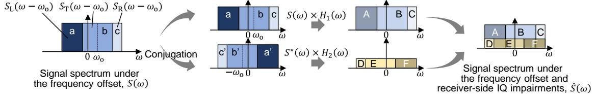
Fig. 2: Crosstalk occurrence process due to the interaction between the frequency offset and receiver-side IQ impairments.
