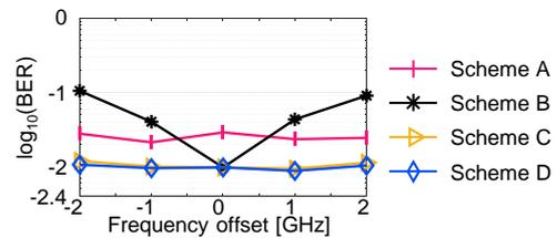
Fig. 7: Measured frequency offset tolerance without IQ impairments.
