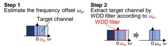
Fig. 1: Concept of the frequency-offset-adaptive WDD.
