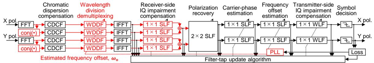
Fig. 6: Configuration of the DSP circuit. (SLF: strictly linear filter and WLF: widely linear filter).
