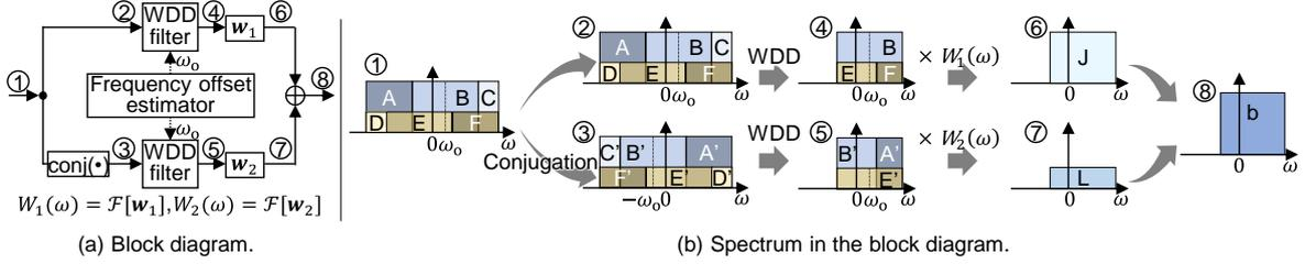
Fig. 4: Proposed process of WDD and WL equalization.
