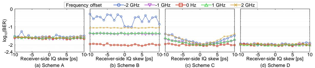
Fig. 8: Measured tolerance for receiver-side IQ impairments and the frequency offset.
